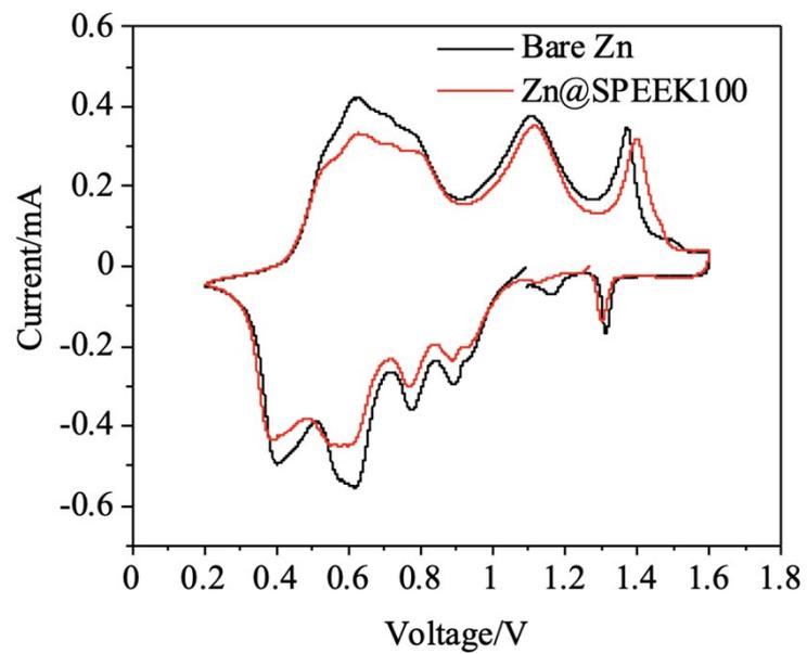
Figure S13 CV profiles of bare zinc and Zn@SPEEK100 in full cell
