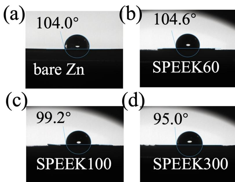
Figure S6 Contact angle of (a) bare zinc, (b) Zn@SPEEK60, (c) Zn@SPEEK100, and (d) Zn@SPEEK300
