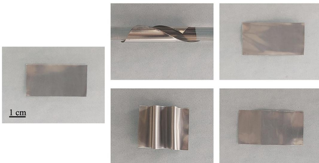
Figure S5 Bending and twisting of Zn@SPEEK100
