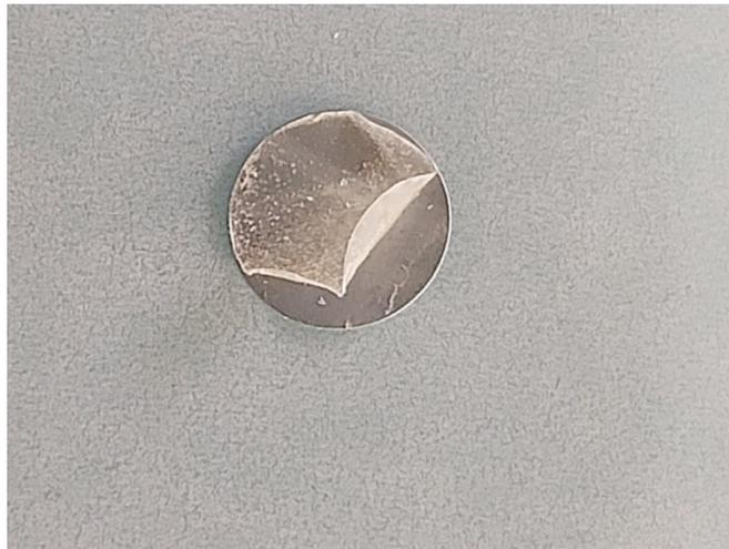
Figure S11 Swelling and peeling off of SPEEK300 membrane
