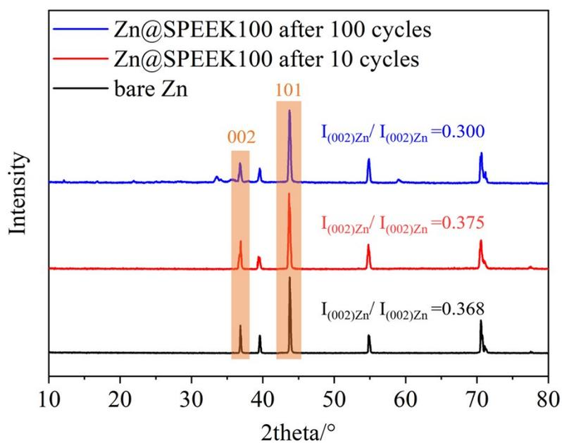
Figure S10 XRD profiles of pristine zinc and Zn@SPEEK100 after cycles
