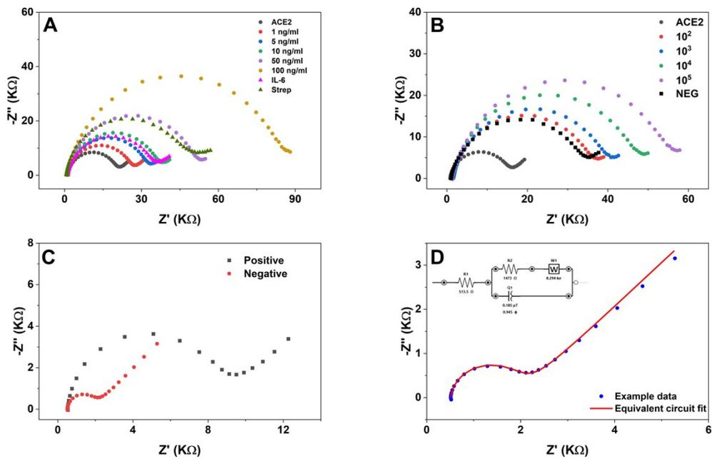
**Figure S3. Showing example Nyquist plots for: Spike protein concentrations, IL-6 and streptavidin (A). Various inactivated virus concentrations plus negative control (B). Positive and negative VPSS clinical samples (C). Example Nyquist data fitted using R[(RW)Q] equivalent circuit parameters (D). This circuit was used to fit all data.**
