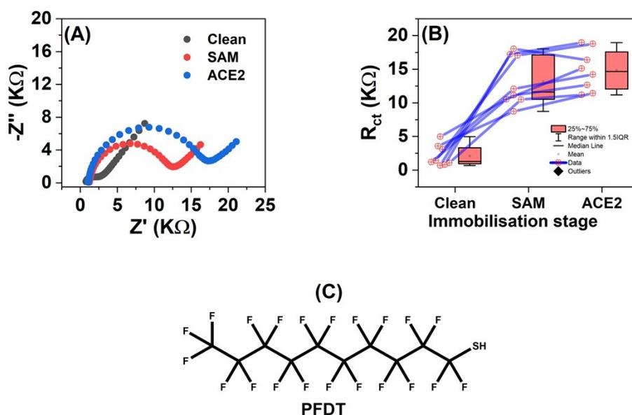
Figure S1. (A) Example Nyquist plots from a representative electrode following cleaning (black), PFDT functionalisation (red) and ACE2 incubation (blue). (B) Box plot showing  $R_{ct}$  values through the three stages of electrode functionalisation (cleaning, SAM formation and ACE2 immobilisation). (C) Structural formula of PFDT.
