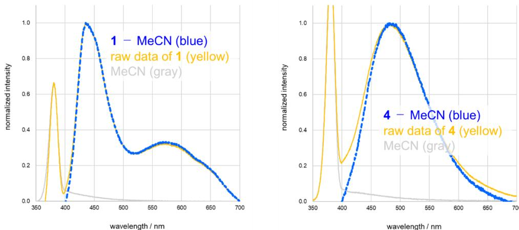
**Figure S6.** Fluorescence emission spectra of **1** and **4** in MeCN ( $5.0 \times 10^{-4}$  M) (blue: after removal of background, yellow: raw data, gray: solvent only)
