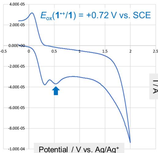
**Figure S4.** Cyclic voltammogram of **1** in 100 mM TBAP/MeCN
