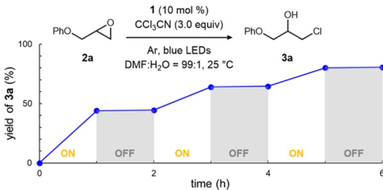
**Figure S2.** ON/OFF experiments
