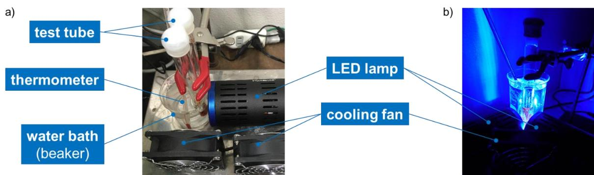
**Figure S1.** Equipment for photoredox reactions by **1** (a: 0.2 mmol scale, b: 1.0 mmol scale)
