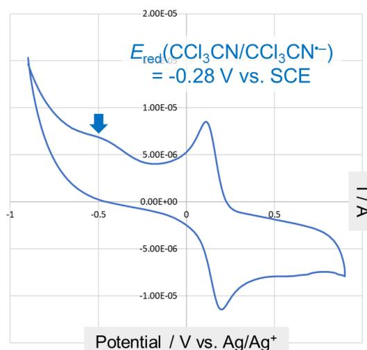
**Figure S5.** Cyclic voltammogram of CCl<sub>3</sub>CN in 100 mM TBAP/MeCN
