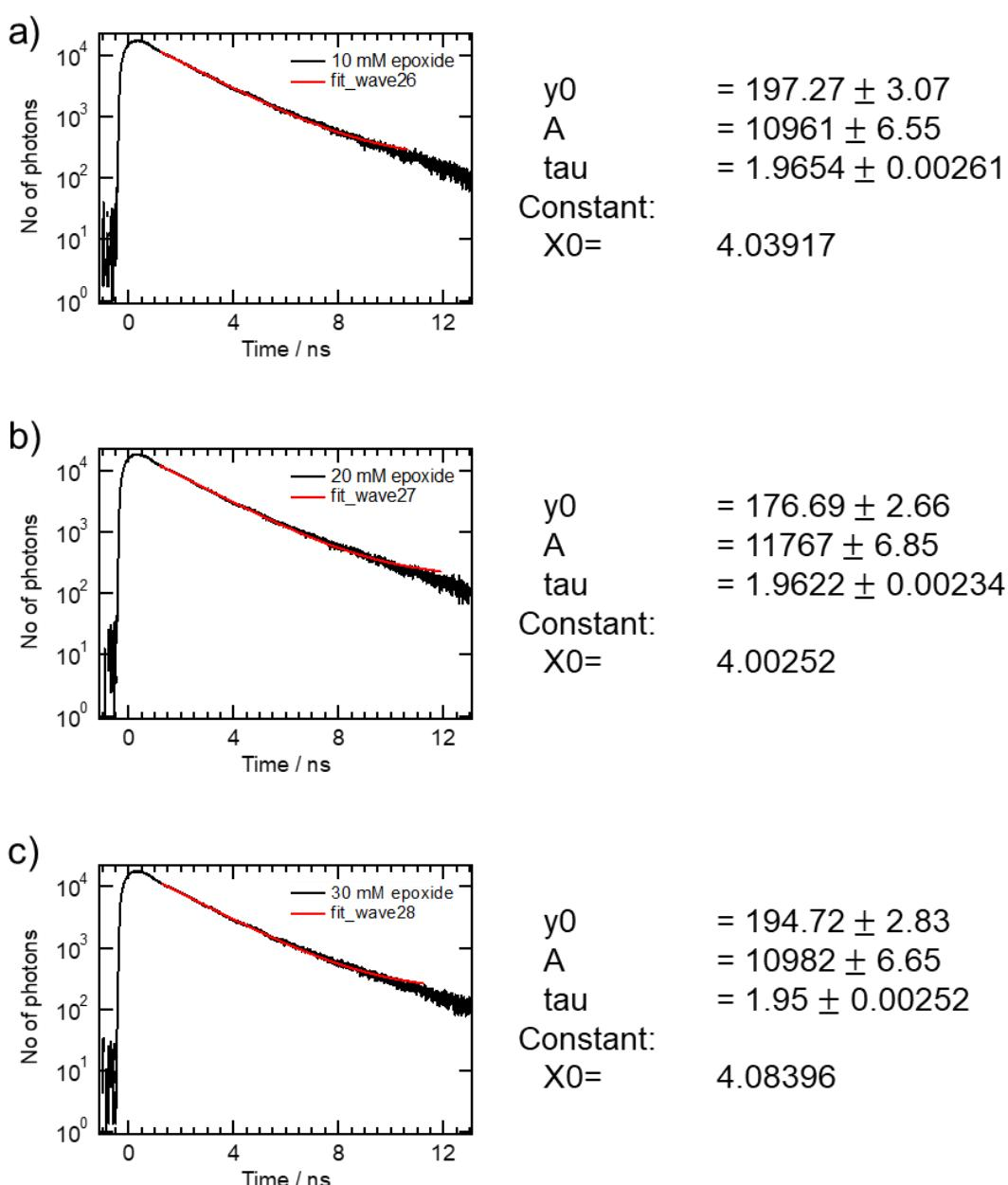
**Figure S12.** Fluorescence intensity decay profiles
