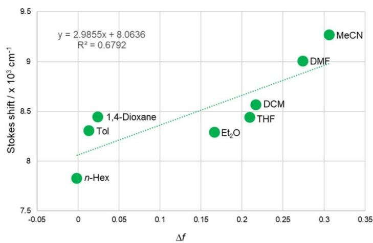
**Figure S7.** Lippert–Mataga plot of **1**:  $\Delta f = [(\varepsilon - 1)/(2\varepsilon + 1)] - [(n^2 - 1)/(2n^2 + 1)]$  ( $\varepsilon$ : dielectric permittivity of the solvent,  $n$ : refractive index of the solvent)
