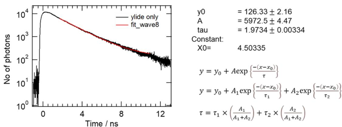
**Figure S10.** Fluorescence intensity decay profile of phosphonium ylide **1**
