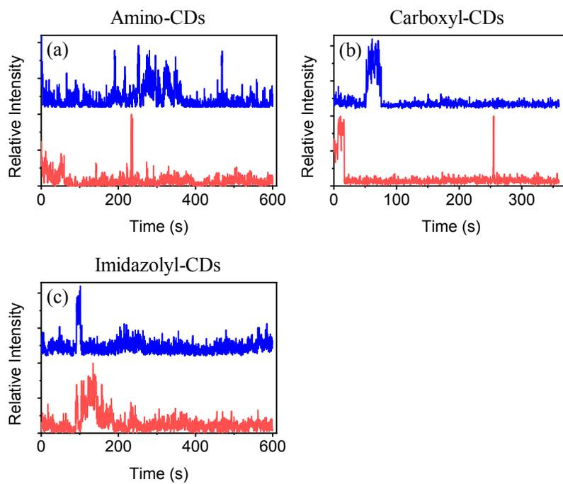
**Fig. S9** Single particle intensity trajectories for different CDs. Two random intensity trajectories change over time for single (a) Amino-CDs, (b) Carboxyl-CDs, (c) Imidazolyl-CDs. All CDs were excited with 532 nm laser. Exposure time were 287 ms.
