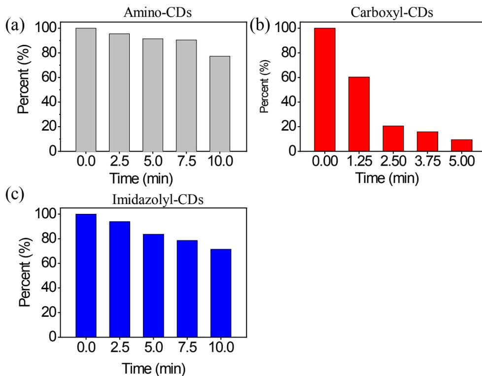
**Fig. S11** Number fraction of different CDs during continuous illumination. (a) Amino-CDs number change over time, (b) Carboxyl-CDs number change over time, (c) Imidazolyl-CDs number change over time. All CDs were excited with 532 nm laser. The number of CDs on  $256 \times 256$  pixels<sup>2</sup> region was counted and normalized as a function of illumination time. Exposure time were 287 ms.
