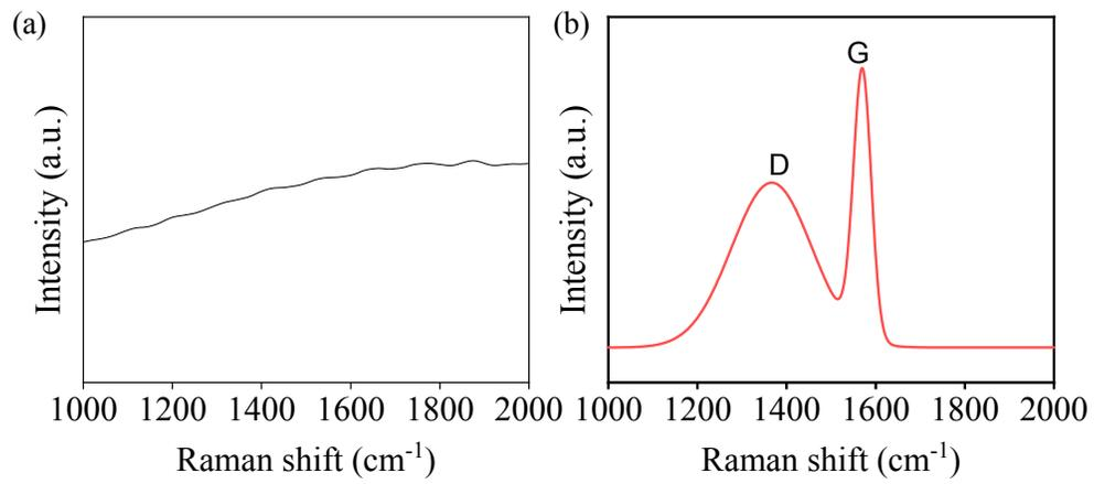
**Fig. S4** Raman spectra of (a) CA-EDA CDs and (b) our CDs.
