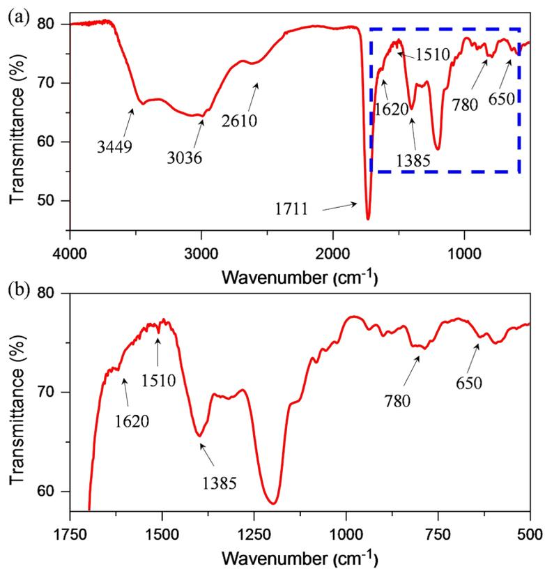
**Fig. S2** (a) FTIR spectrum of CDs and (b) the enlarged view of the region as marked in (a).
