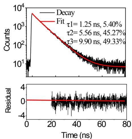
**Fig.S7** Fluorescence decay curves (black) and fitted curves (red) of DBP-CDs, excited at 532 nm. The decay curves were fitted to a triexponential decay function. The average lifetime was calculated by using the equation,  $\tau = A_1\tau_1 + A_2\tau_2 + A_3\tau_3$ .  $A_1$ ,  $A_2$ , and  $A_3$  are the fractional contributions of the lifetime components  $\tau_1$ ,  $\tau_2$ , and  $\tau_3$ .
