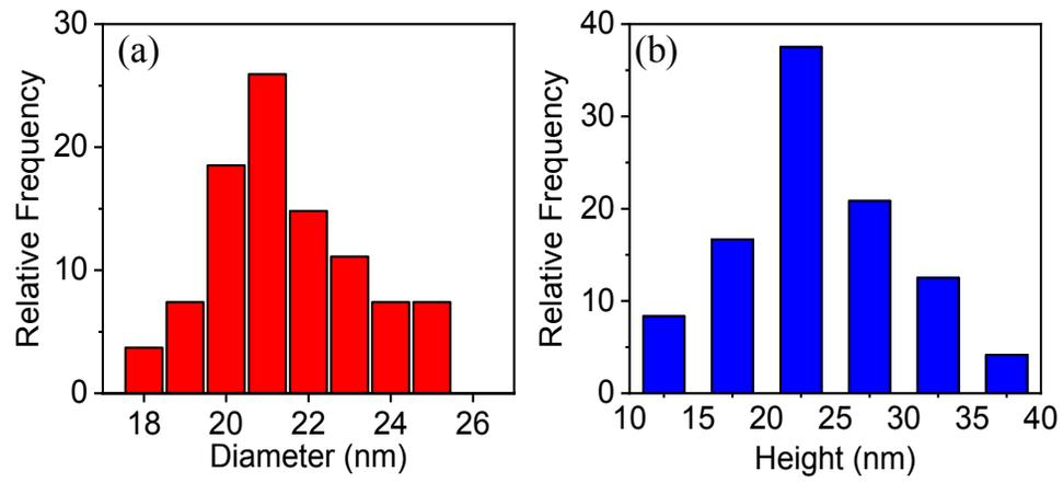
Fig. S1. The size or height distribution of CDs determined from (a) TEM and (b) AFM images.
