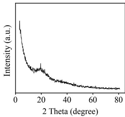
**Fig. S3** XRD profile of DBP-CDs.
