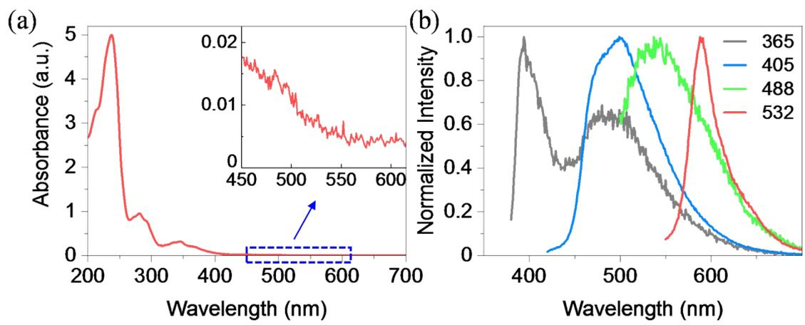
**Fig. S6** (a) UV-Vis absorption and the enlarged view of the region (inset) and (b) normalized fluorescence spectra of CDs excited at different wavelengths.
