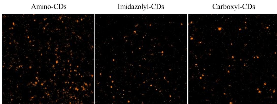
**Fig. S8** Single molecule fluorescence imaging of different commercial CDs by TIRFM, (a) Amino-CDs, (b) Carboxyl-CDs, (c) Imidazolyl-CDs. Exposure time: 287 ms/frame. Excitation laser: 532 nm.
