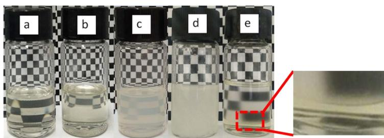
**Figure S4.** Emulsions photographs with aqueous phase contents (mg/mL): a) 0; b) 26; c) 74; d) 84; e) 224, 1-pentanol and aqueous phase were separated.
