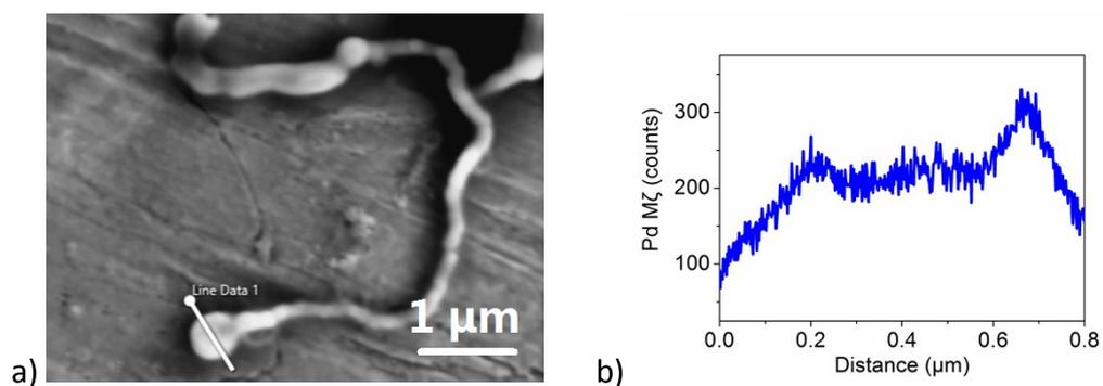
**Figure S13.** The SEM image (a) and EDX elemental line-scan profile (b) of the tadpole-like Janus Pd-nanotubes.
