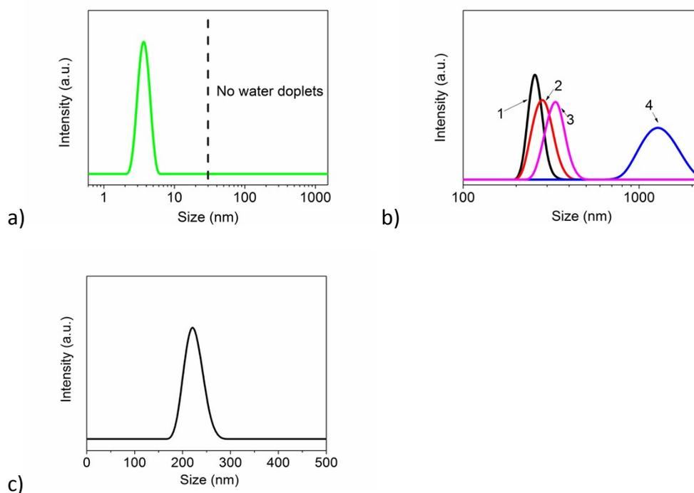
**Figure S3.** DLS size analysis of 1-pentanol solution of PVP (a) and the water droplets in the water in 1-pentanol emulsion with different aqueous phase contents (mg/mL) (b): line 1) 26; line 2) 34; line 3) 59; line 4) 84; the water droplets in 1-pentanol phase when 224 mg/mL aqueous phase contents is used (the upper 1-pentanol phase) (c).
