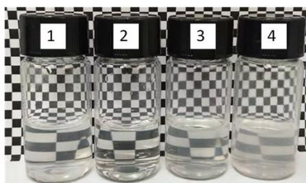
**Figure S11.** Dispersions photographs of the tadpole-like Janus nanotubes (1, 3) and the tadpole-like nanotubes (2, 4) in water (1, 2) or hexane (3, 4).
