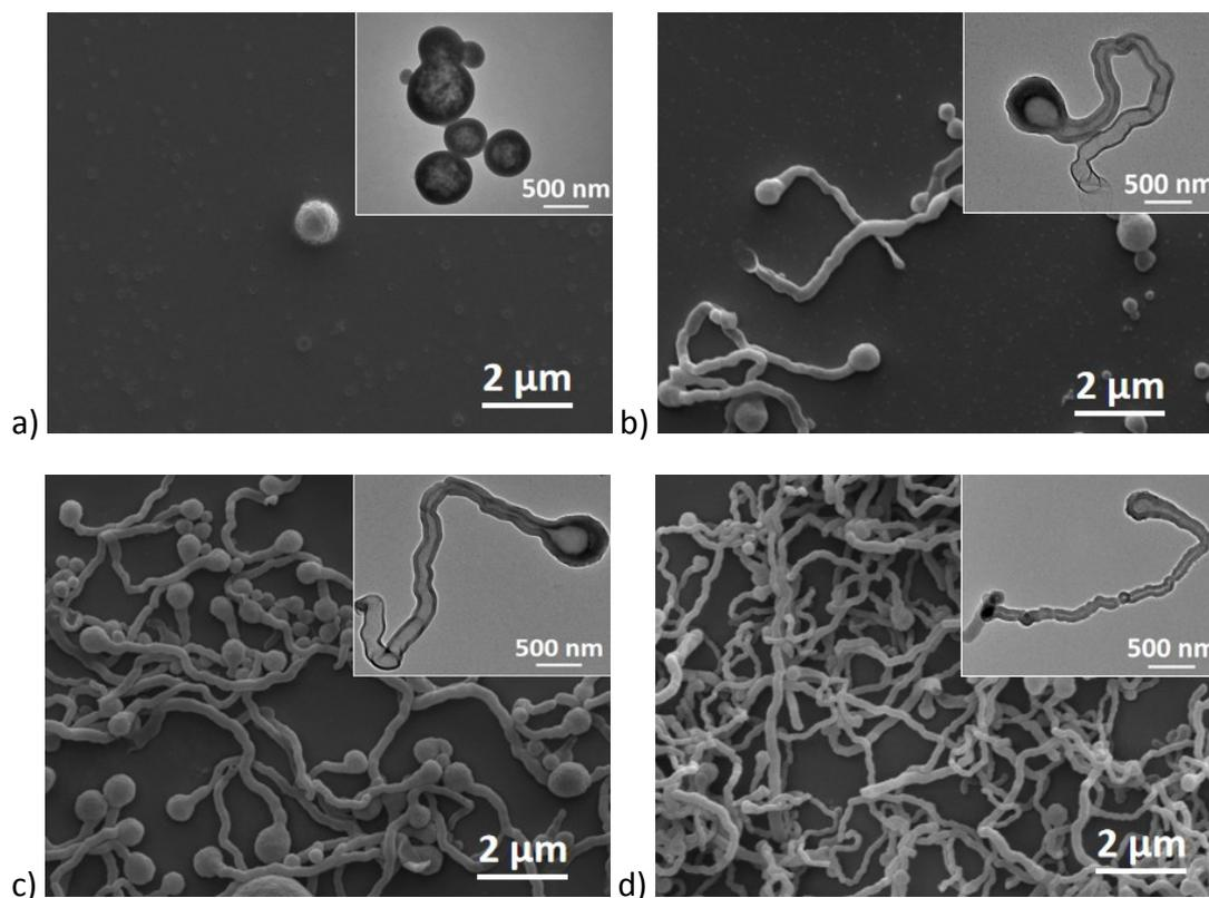
**Figure S7.** SEM and inset TEM images of the tadpole-like nanotubes with different  $\text{NH}_4\text{OH}$  concentration in the aqueous phase (mmol/L): a) 0; b) 8.71; c) 17.42; d) 226.46.
