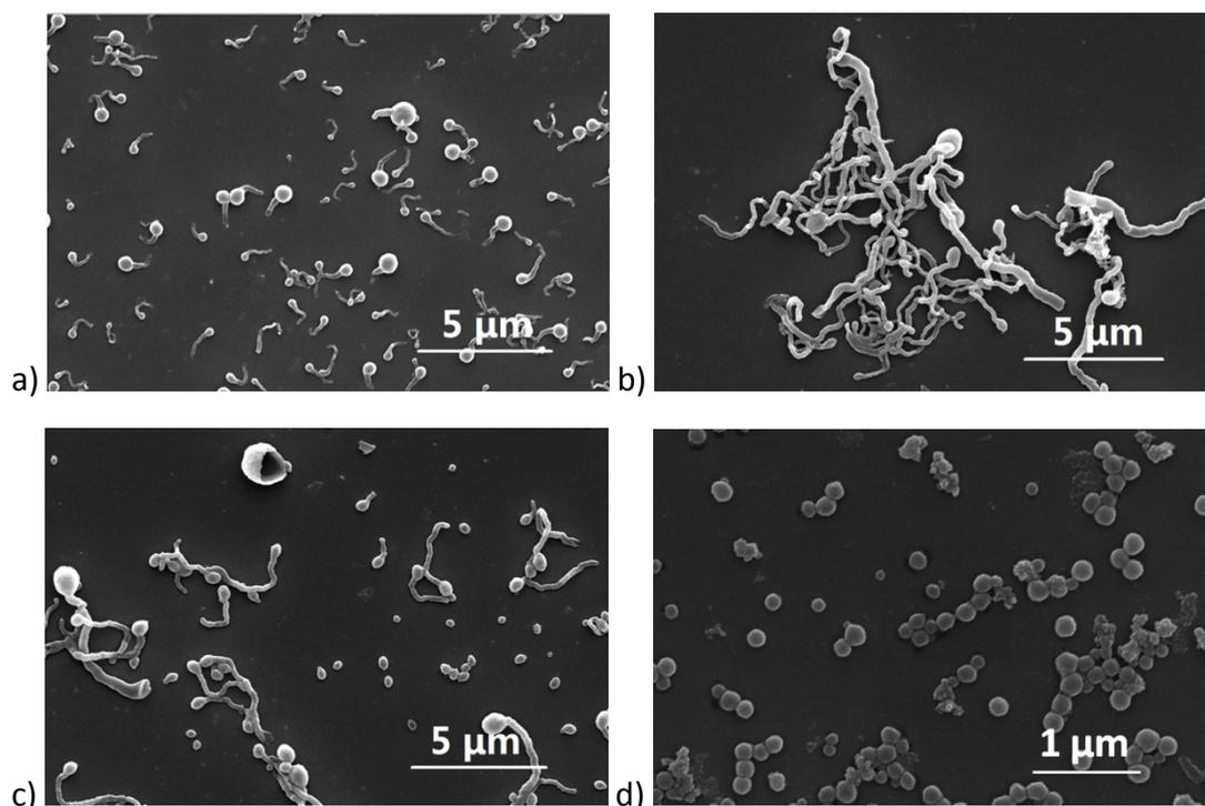
**Figure S2.** SEM images of the tadpole-like nanotubes with different aqueous phase contents (mg/mL): a) 29; b) 59; c) 74; d) 224. The  $\text{NH}_4\text{OH}$  concentration in the aqueous phase is 122 mmol/L, and the reaction time is 24 h.
