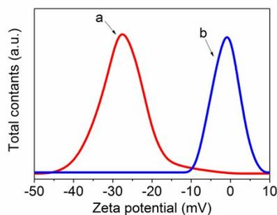
**Figure S12.** Zeta potential of the tadpole-like nanotubes (line a) and the tadpole-like Janus nanotubes (line b).
