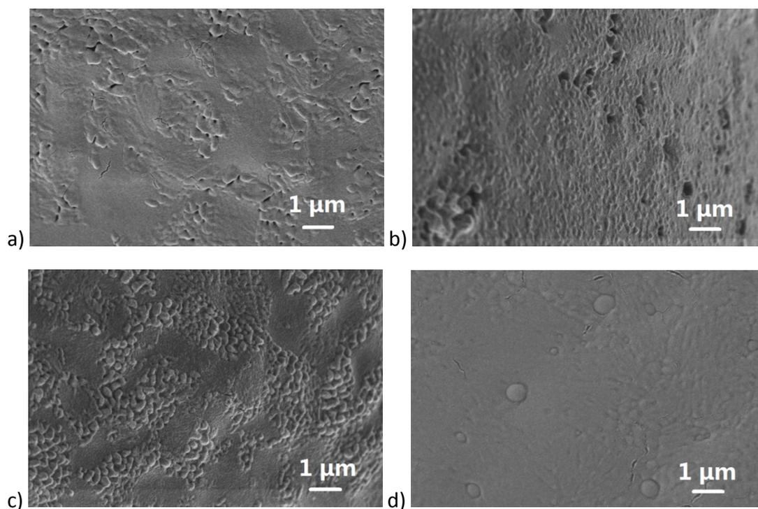
**Figure S5.** Cryo-SEM images of emulsions with aqueous phase contents (mg/mL): a) 26; b) 34; c) 59; d) 84.
