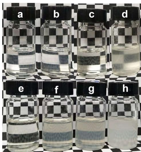
**Figure S8.** Emulsions photographs of the tadpole-like nanotubes with different  $\text{NH}_4\text{OH}$  concentration in the aqueous phase (mmol/L): a, e) 0; b, f) 8.71; c, g) 17.42; d, h) 226.46. The aqueous phase content is 59 mg/mL, and the reaction time is 24 h (a-d) and 72 h (e-h), respectively.
