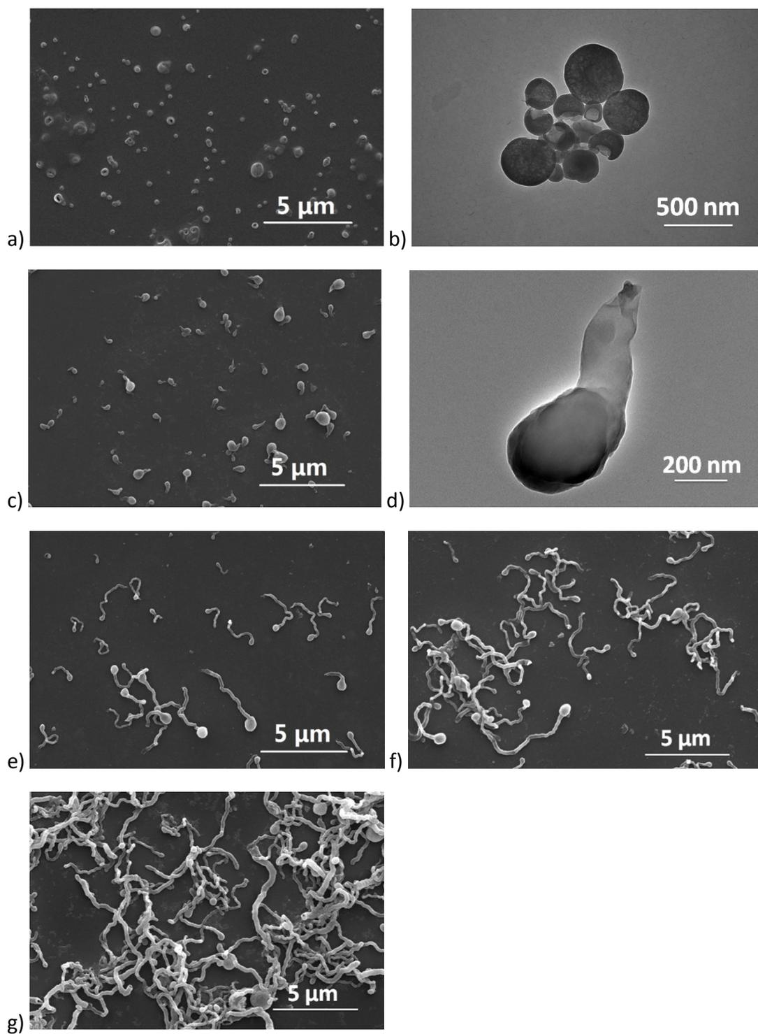
**Figure S1.** SEM and TEM images of the tadpole-like nanotubes with different reaction time (h): a, b) 0.5; c, d) 1; e) 5; f) 16; g) 48. The aqueous phase content is 59 mg/mL, and the  $\text{NH}_4\text{OH}$  concentration in the aqueous phase is 122 mmol/L.
