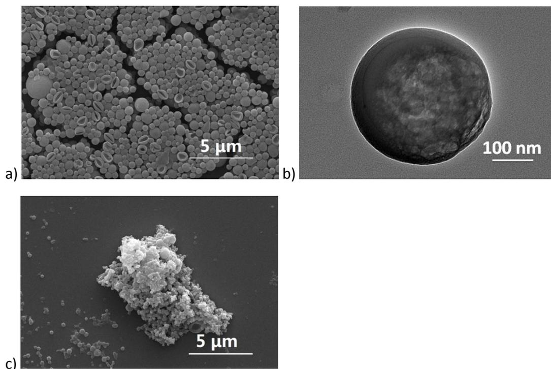
**Figure S10.** SEM and TEM images of the tadpole-like nanotubes with different HCl concentration in the aqueous phase (mmol/L): a, b) 9.66; c) 228.26. The aqueous phase content is 59 mg/mL, and the reaction time is 24 h.
