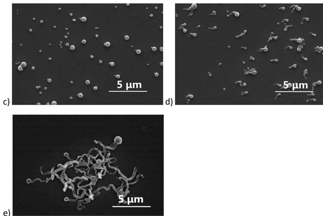
**Figure S6.** SEM and TEM images of the tadpole-like nanotubes with different  $\text{NH}_4\text{OH}$  concentration in the aqueous phase (mmol/L): a, b) 0; c) 8.71; d) 17.42; e) 226.46. The aqueous phase content is 59 mg/mL, and the reaction time is 24 h.
