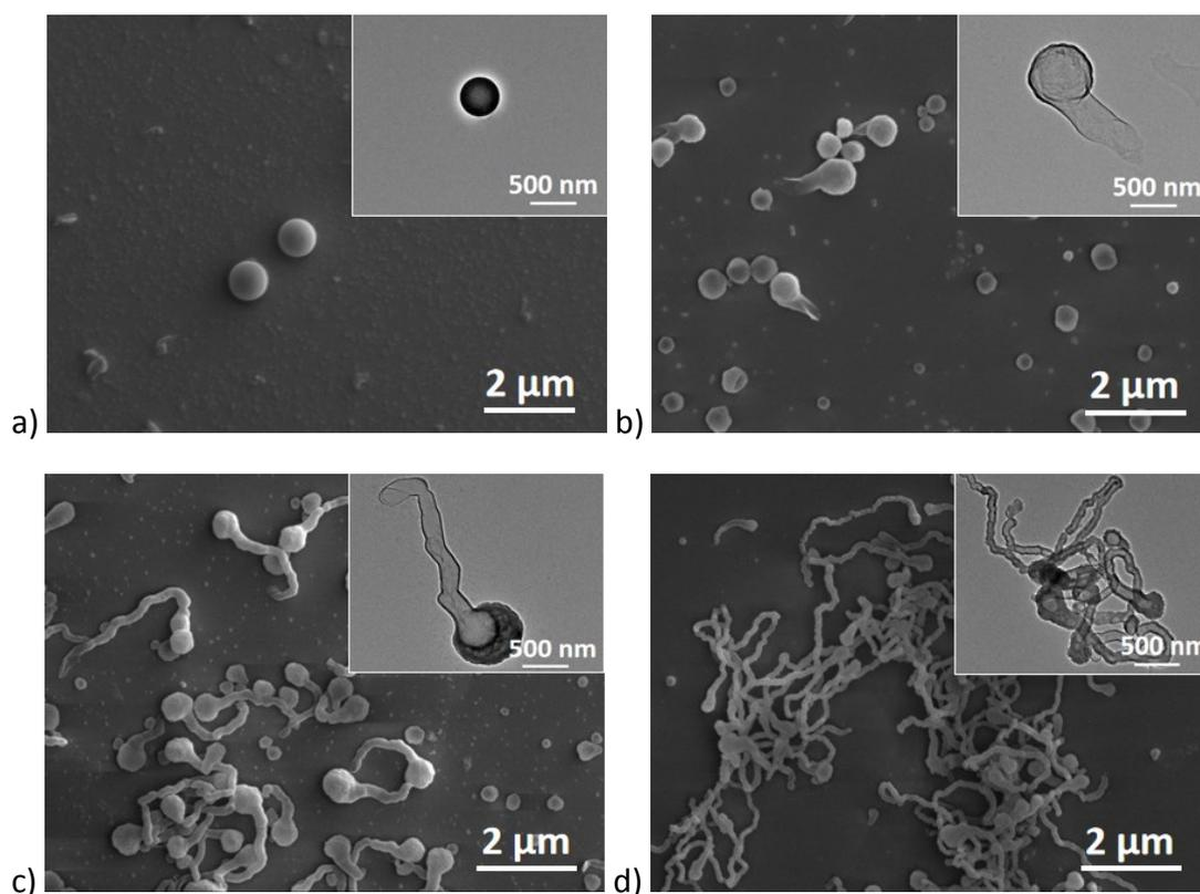
**Figure S9.** SEM and inset TEM images of the tadpole-like nanotubes with different  $\text{NH}_4\text{OH}$  concentration in the aqueous phase (mmol/L): a) 0; b) 8.71; c) 17.42; d) 226.46. The aqueous phase content is 59 mg/mL, the reaction time is 24 h, and the temperature is 40 °C.
