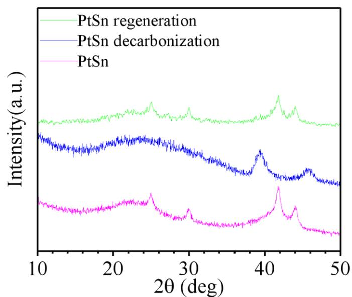
**Figure S5.** PXRD of pristine PtSn@mSiO<sub>2</sub> and that after decarbonization and regeneration processes.
