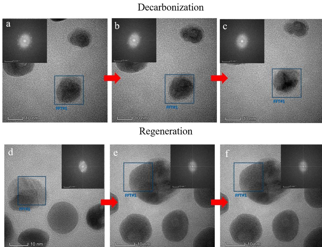
**Figure S2.** TEM images of PtSn@mSiO<sub>2</sub> nanoparticles after decarbonization (a-c) and regeneration (d to f) treatments. The corresponding FFT patterns of the selected areas are shown as insets.
