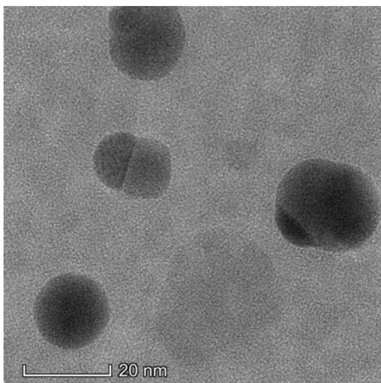
**Figure S3** TEM images of PtSn@mSiO<sub>2</sub> when heated under 760 torr pure oxygen at 500°C.
