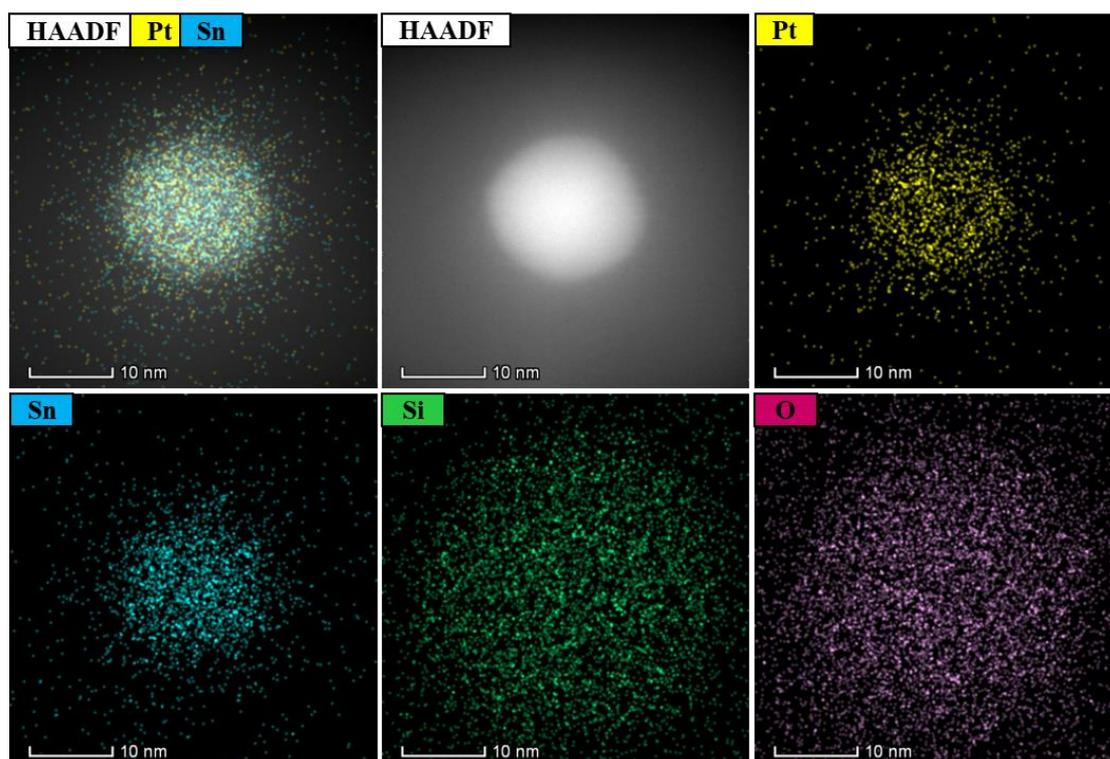
**Figure S6.** HAADF-STEM elemental distribution of initial state PtSn@mSiO<sub>2</sub> iNPs. Pt: yellow; Sn: blue; Si: green; O: purple.
