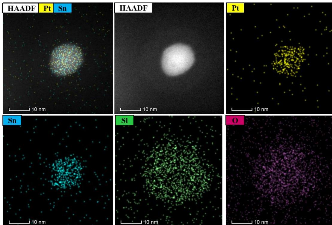
**Figure S8.** HAADF-STEM elemental distribution of after regeneration state PtSn@mSiO<sub>2</sub> iNPs. Pt: yellow; Sn: blue; Si: green; O: purple.
