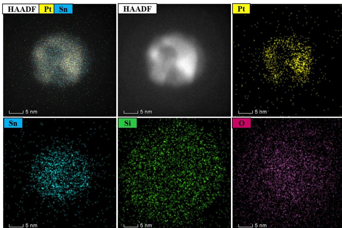
**Figure S7.** HAADF-STEM elemental distribution of after deactivation state PtSn@mSiO<sub>2</sub> iNPs. Pt: yellow; Sn: blue; Si: green; O: purple.
