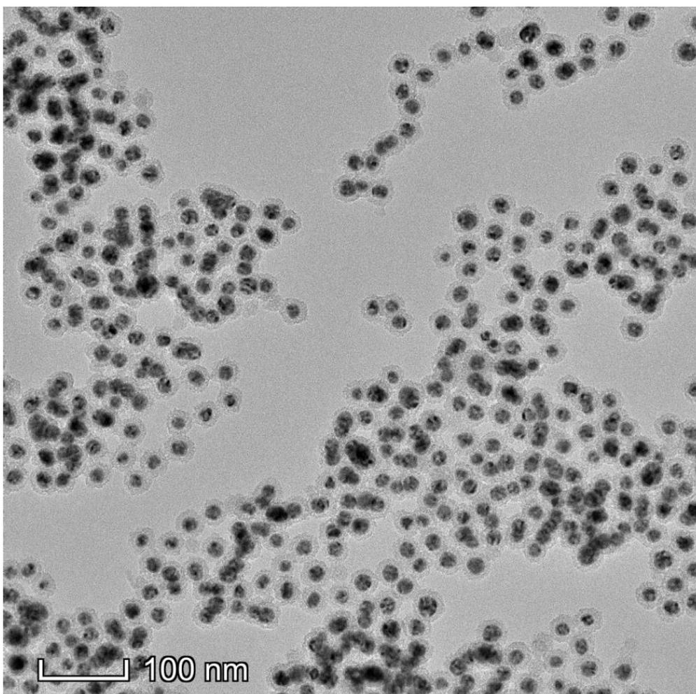
**Figure S1:** PtSn@mSiO<sub>2</sub> nanoparticles after being heated at 500°C in air for 4h.
