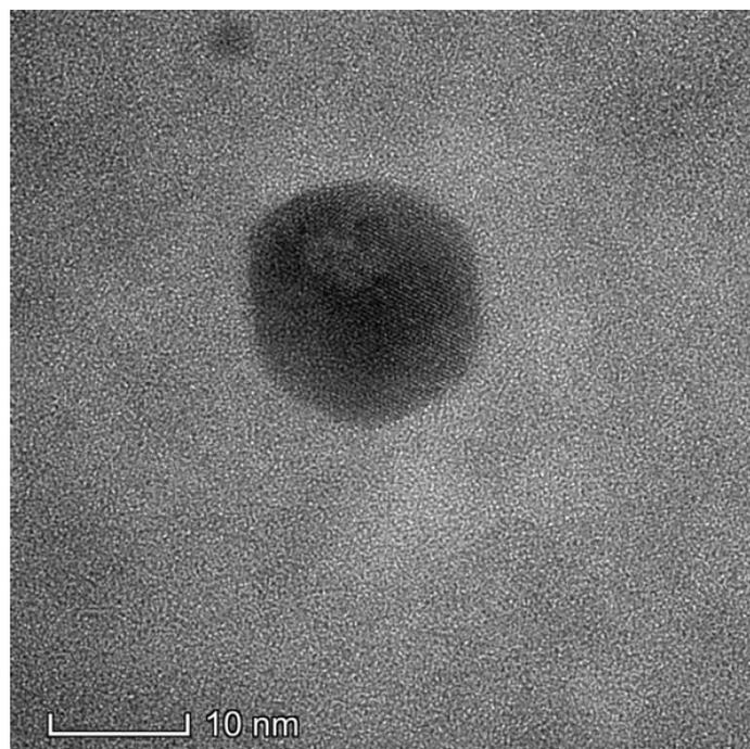
**Figure S4** High-magnification TEM image of one PtSn@mSiO<sub>2</sub> nanoparticle after regeneration process. The nanoparticle regains its regular shape and ordered crystal structure.
