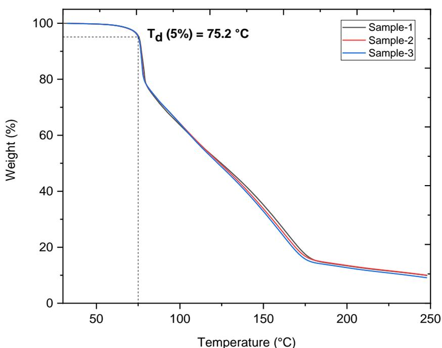
**Figure S7.** The TGA curve of *N*-transfer reagent D7.
