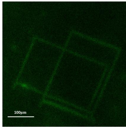
**Fig. S6** single photon lithography. One layer is printed by focusing a CW laser (405 nm) on the surface of the film and another layer is printed by focusing the laser at 50µm below the surface, but the created two layers overlap in the z direction, which suggests poor printing resolution in the z direction by single photon lithography.
