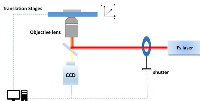
Fig. S3 The illustration of the optical setup.
