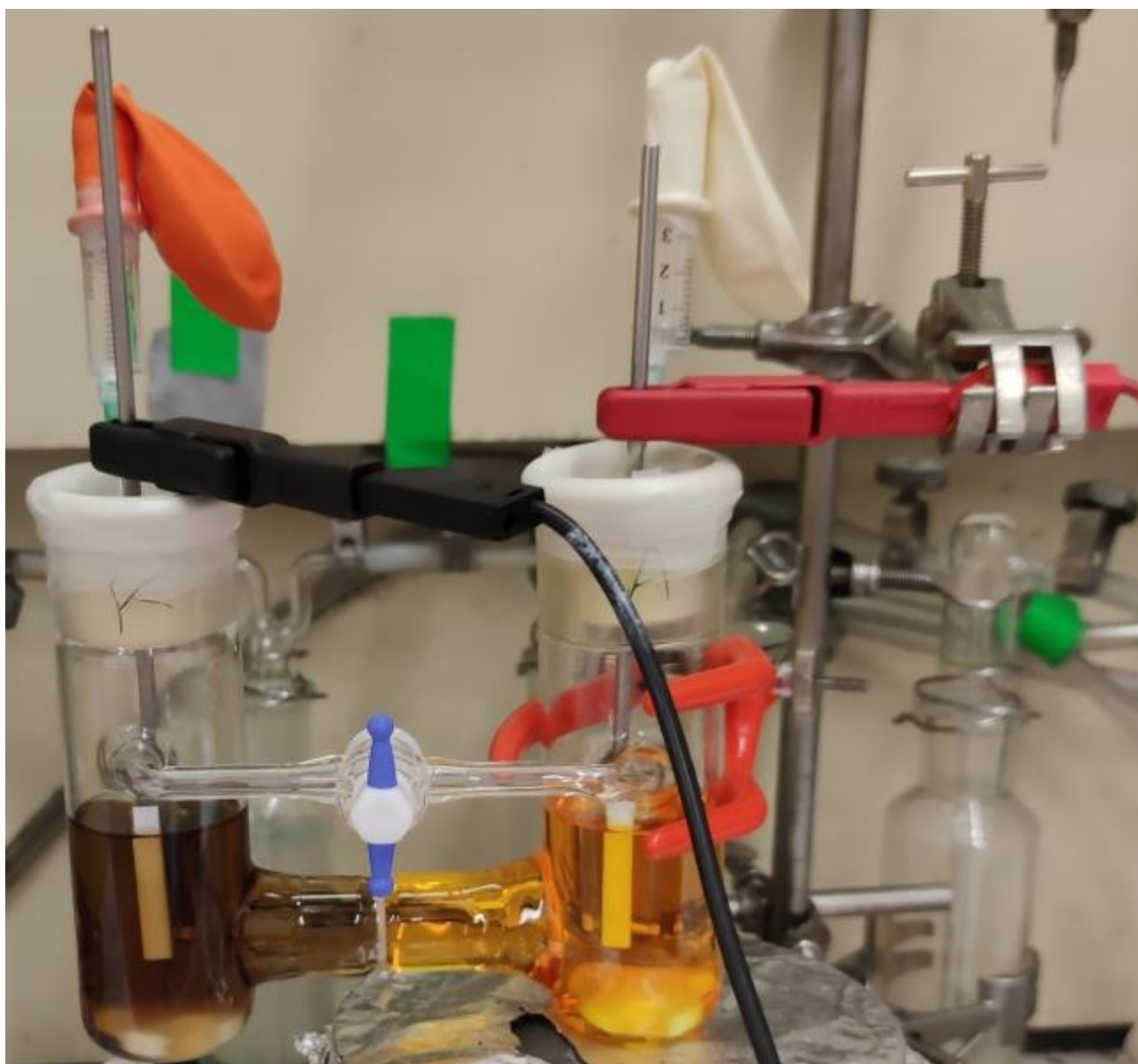
Figure 4. H-type divided glass cell during electrolysis.
