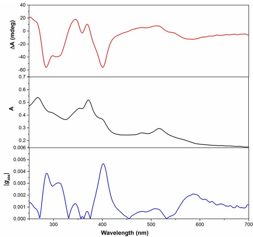
**Figure S13.** Circular dichroism (top) and absorption (middle) spectra as well as the absolute absorption dissymmetry factor ( $|g_{abs}|$ ) curve (bottom) of the drop-casted thin film of (*M,M*)-**1**. The absorption dissymmetry factor was calculated by  $g_{abs} = \Delta A/A^3$ , where  $\Delta A$  (mdeg) is converted to  $\Delta A$  (a.u.) by  $\Delta A$  (a.u.) =  $\Delta A$  (mdeg) / 32982.
