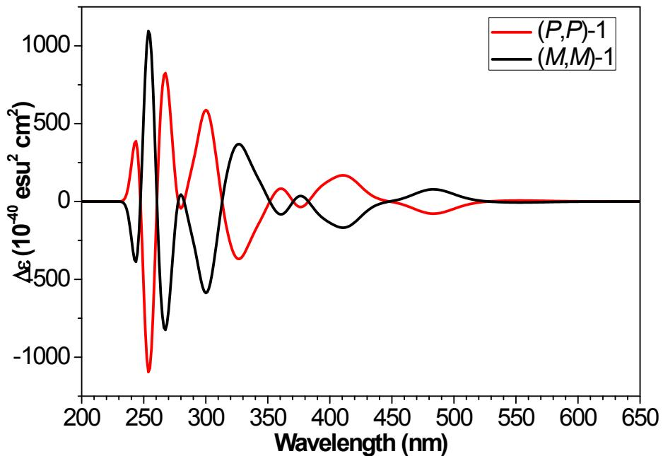
**Figure S12.** Simulated CD spectra of (*P,P*)-**1** and (*M,M*)-**1** by TD-DFT calculation.
