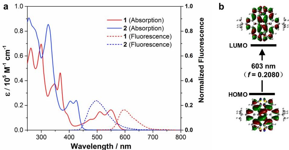
**Figure S11.** (a) UV-Vis absorption (solid lines) and emission (dotted lines) spectra of compounds **1** and **2** in chloroform with the concentration of  $1 \times 10^{-5} \text{ M}$ . (b) the molecular orbitals and electronic transition diagram of **1**.
