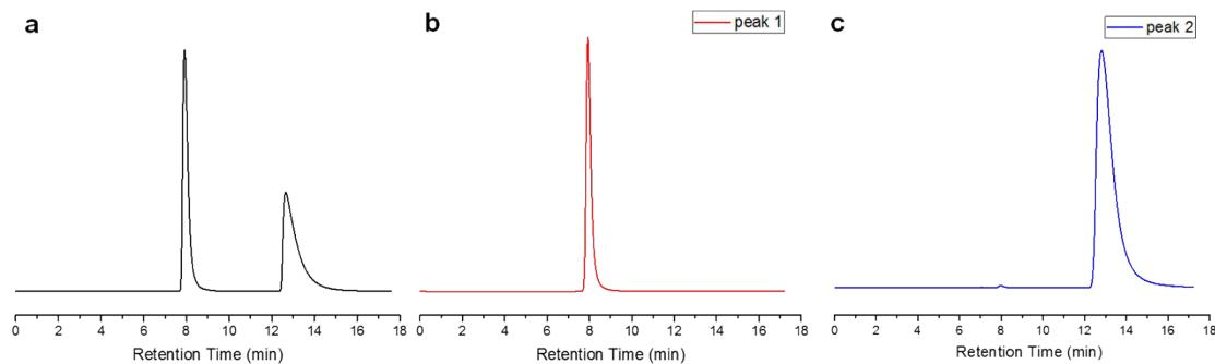
**Figure S1.** Chiral HPLC traces for the separation of racemic **1** (a), the first eluting enantiomer (b) and the second eluting enantiomer (c) using chloroform as eluent with a flow rate of 0.5 mL/min.
