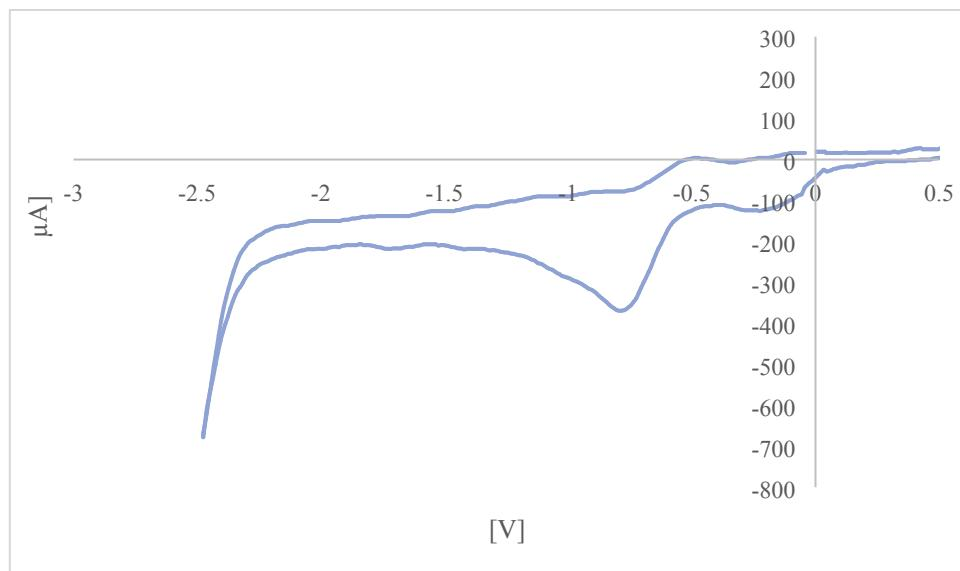
Figure S159. Cyclic voltammetry measurement of lutidine-mentol-salt **3** in TBA.BF<sub>4</sub> solution (0.1 mM)
