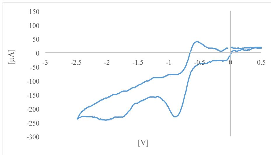
Figure S157. Cyclic voltammetry measurement of control TBA.BF<sub>4</sub> solution (0.1 mM)
