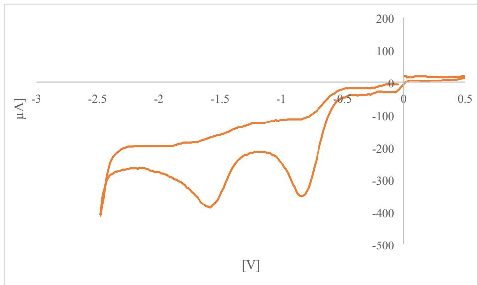
Figure S158. Cyclic voltammetry measurement of compound **2e** in TBA.BF<sub>4</sub> solution (0.1 mM)
