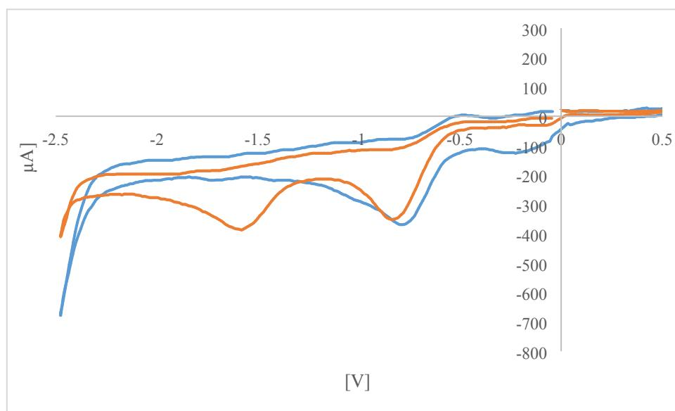
Figure S160. Cyclic voltammetry comparison of **2e** e lutidine-mentol-salt **3** in TBA.BF<sub>4</sub> solution (0.1 mM)
