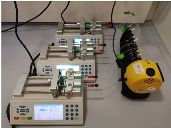
Figure S1. Reaction set-up for the enzymatic epoxidation of *cis*- $\beta$ -methylstyrene. On the left, syringe pumps for continuous  $^t\text{BuOOH}$  supply. Syringes are connected to tubes which lead to the reaction mixture inside GC vials on the right. An overhead rotator is used for shaking of the reaction at 99 rpm, 60 ° at room temperature.
