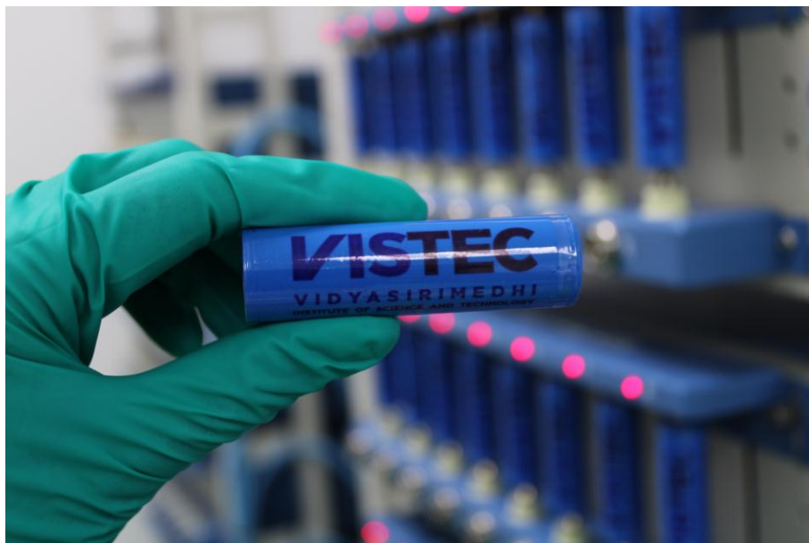
Figure S10. As-fabricated cylindrical 18650-type lithium-ion battery.
