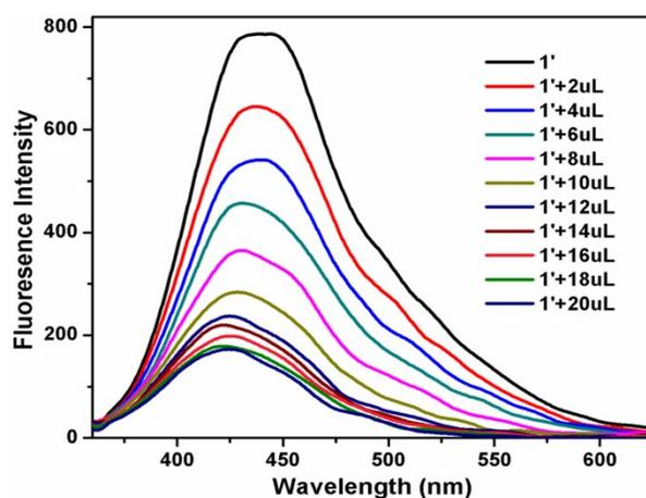
**Fig. S13** Change of fluorescence intensity of **1'** upon addition of Pd<sup>2+</sup> at an emission slit of 9 nm [all spectra were acquired at room temperature at excitation slit 340 nm].
