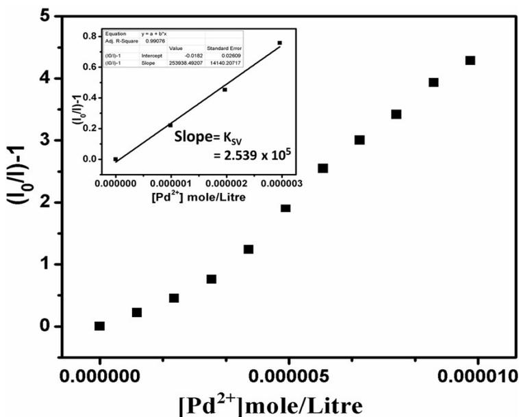
**Fig. S15** Plot of the quenching efficiency of **1'** dispersed in H<sub>2</sub>O upon the addition of different concentrations of Pd<sup>2+</sup>. Inset shows the linear relationship between  $(I_0/I) - 1$  and concentration.
