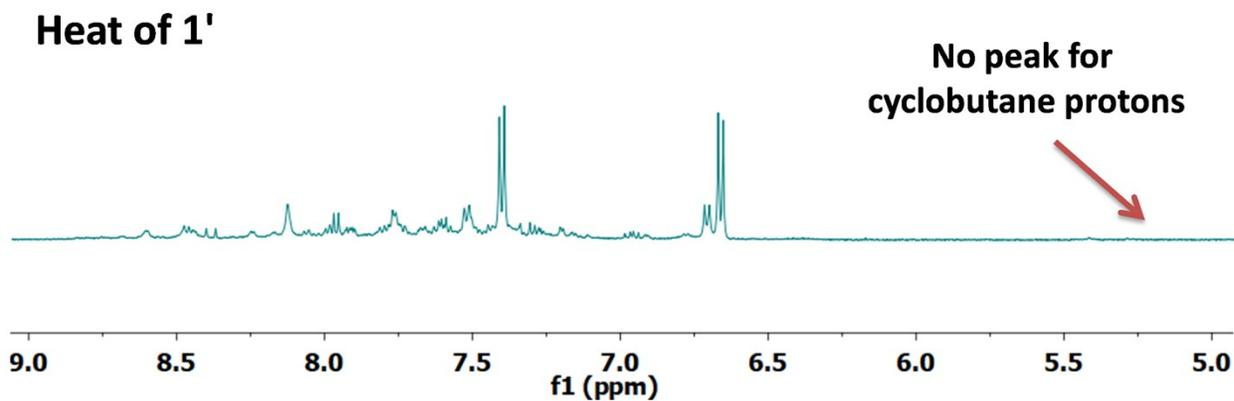
**Fig. S10** Partial  $^1\text{H}$  NMR spectra (400 MHz,  $\text{DMSO-d}_6$ ) of heated **1'** at 200 °C.
