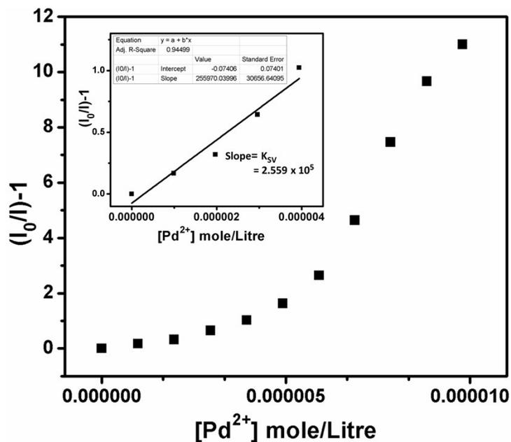
**Fig. S14** Plot of the quenching efficiency of **1** dispersed in H<sub>2</sub>O upon the addition of different concentrations of Pd<sup>2+</sup>. Inset shows the linear relationship between  $I_0/I - 1$  and concentration.
