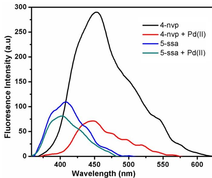
**Fig. S20** Fluorescence spectra of components ligands and also in the presence of Pd<sup>2+</sup> in H<sub>2</sub>O.
