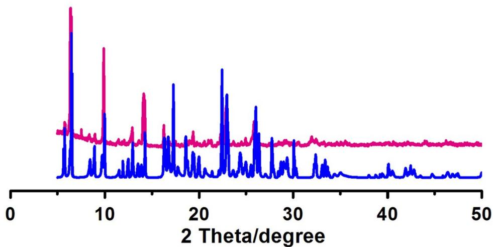
**Fig. S11** PXRD patterns of a) as-synthesized **1** (blue) and b) heated **1'** (pink).
