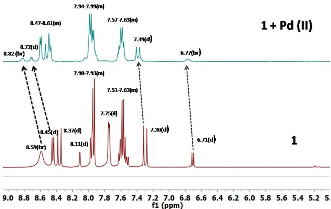
Fig. S21 Partial  $^1\text{H}$  NMR spectra (400 MHz,  $\text{DMSO-d}_6$ ) of compound **1** and **1** with  $\text{Pd}^{2+}$ .
