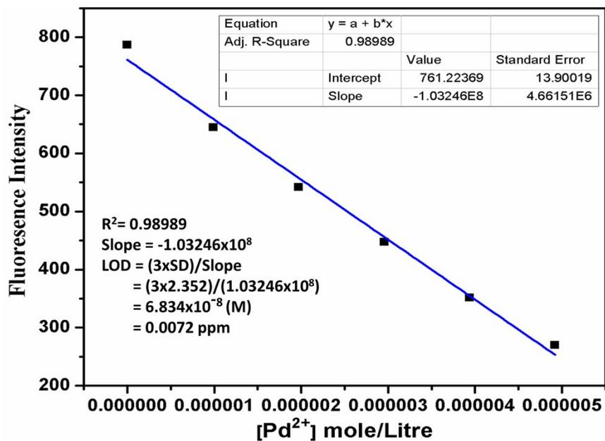
**Fig. S17** The linear dynamic response of compound **1'** for Pd<sup>2+</sup> and the determination of the limit of detection (LOD) of Pd<sup>2+</sup>.
