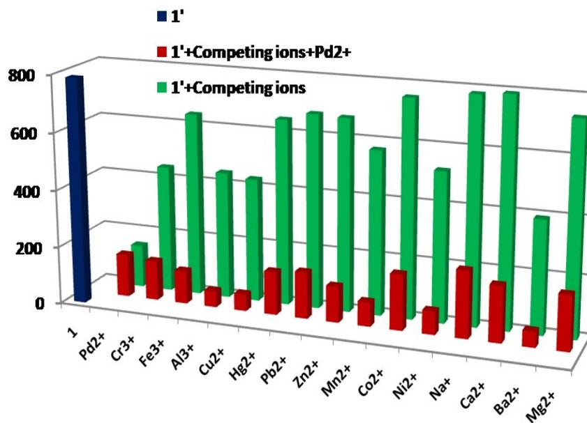
**Fig. S19** Fluorescence intensity of **1'**, its intensity diagram with  $\text{Pd}^{2+}$  along with competing ions and intensity change profile with various competing ions in  $\text{H}_2\text{O}$  medium.
