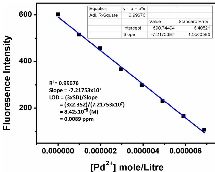
**Fig. S16** The linear dynamic response of compound **1** for Pd<sup>2+</sup> and the determination of the limit of detection (LOD) of Pd<sup>2+</sup>.
