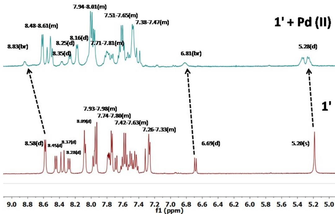
Fig. S22 Partial  $^1\text{H}$  NMR spectra (400 MHz,  $\text{DMSO-d}_6$ ) of compound **1'** and **1'** with  $\text{Pd}^{2+}$ .
