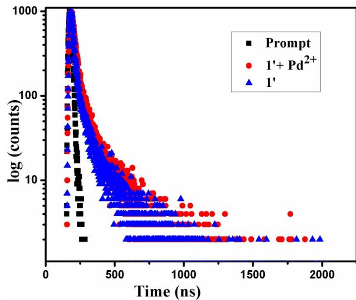
Fig. S24 Excited state decay profile of prompt, compound 1' and compound 1' with Pd<sup>2+</sup> in H<sub>2</sub>O.
