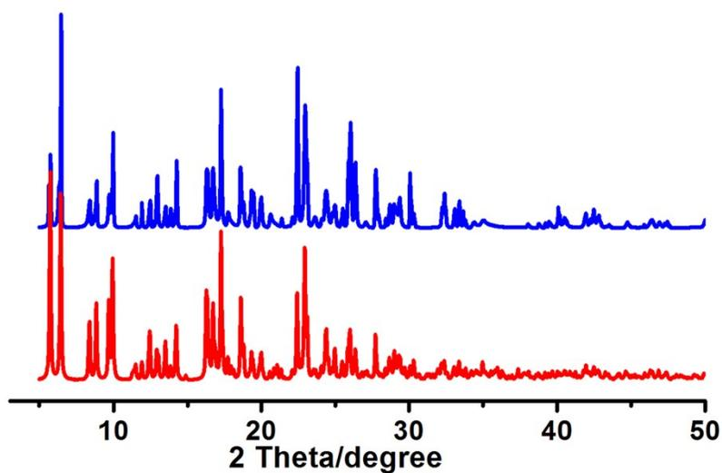
**Fig. S6** PXRD patterns of a) simulated from the X-ray single structure of **1** (red) and b) as-synthesized **1** (blue).
