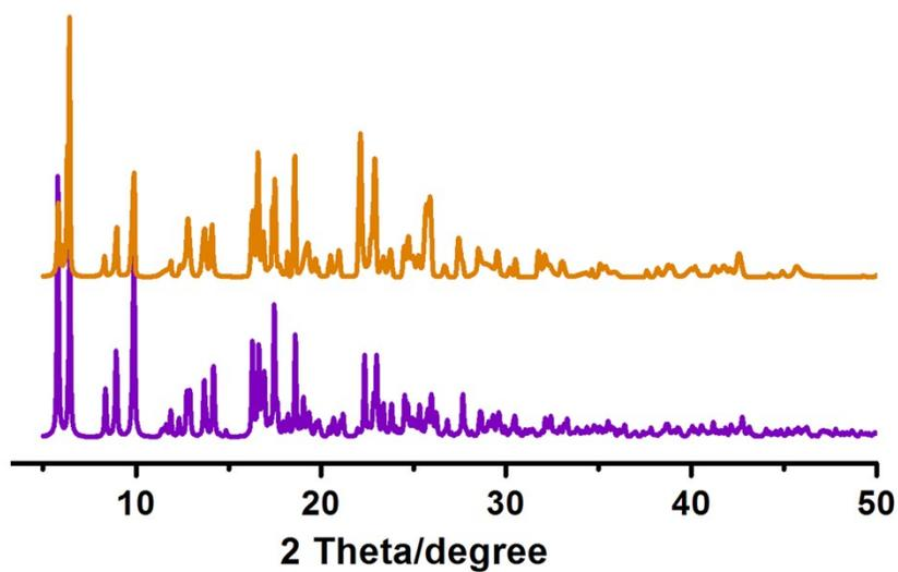
**Fig. S7** PXRD patterns of a) simulated from the X-ray single structure of **1'** (violet) and b) as-synthesized **1'** (light brown).
