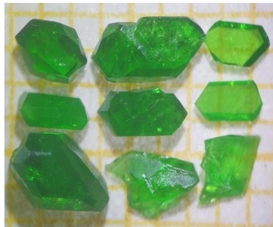
**Fig. S1.** The single crystal of  $\text{CdCu}_2(\text{SeO}_3)_2\text{Cl}_2$ .
