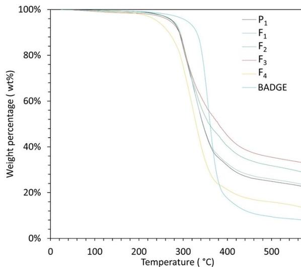
**Figure S28.** TGA thermograms of the cured epoxy networks as function of temperature. The temperature ranged between 20 and 575 °C under N<sub>2</sub> flow (ramp of 10 °C min<sup>-1</sup>).
