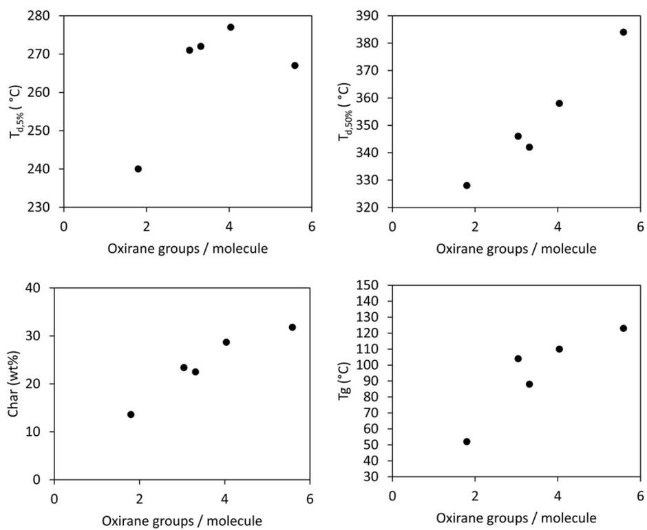
**Figure S30.** Thermal properties of the cured epoxy resins relative to the average number of oxirane moieties per molecule in the respective fractions.
