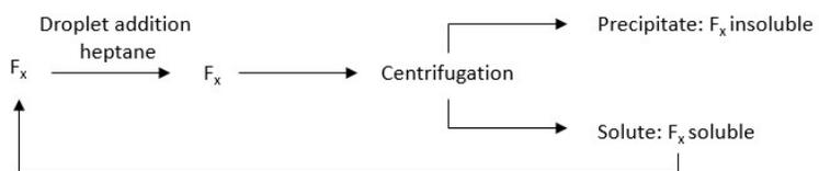
**Figure S1.** Schematic representation of the fractionation based on solvent-anti-solvent precipitation.
