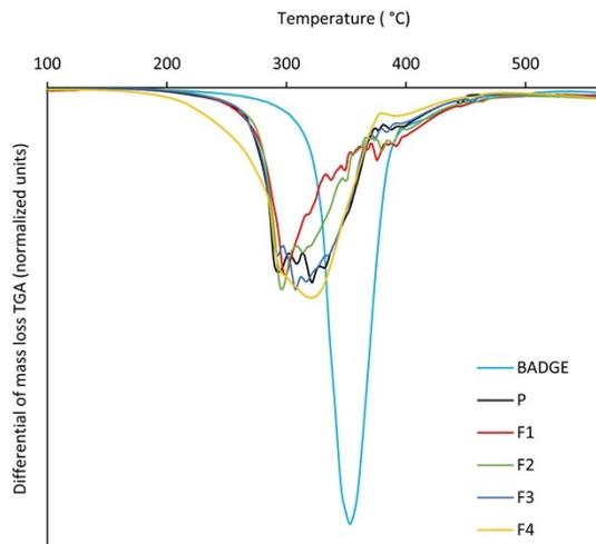
**Figure S29.** DTGA curve of the cured epoxy networks as function of temperature.
