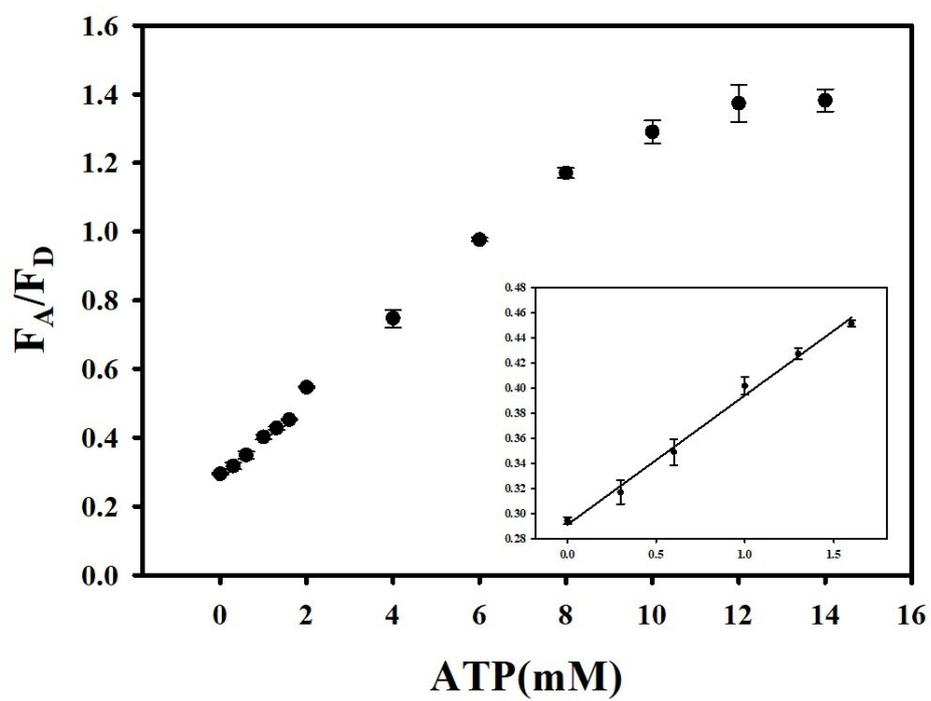
**Figure S2.** A plot of the  $F_A/F_D$  ratio as a function of ATP concentrations. Inset plot is a linear calibration curve of  $F_A/F_D$  ratio as a function of ATP in the lower concentration range.
