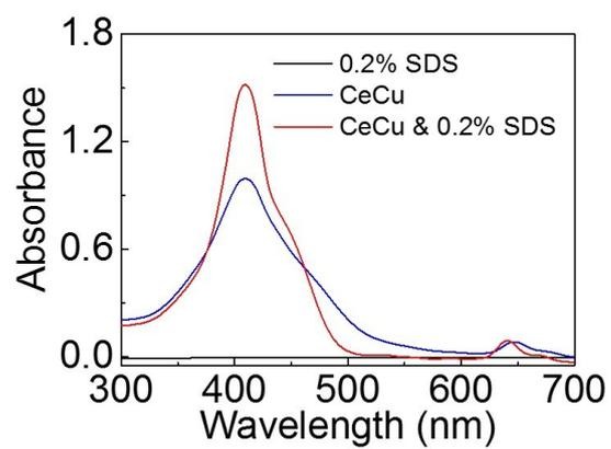
**Fig. S3** The UV-vis spectrum of CeCu in the presence or absence of 0.2% SDS.
