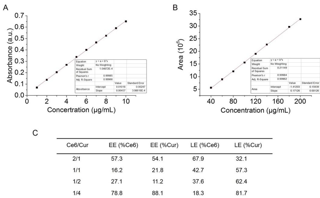
**Fig. S1** Stand curves of (A) Ce6 and (B) Cur detected by UV-vis spectrum and HPLC.
