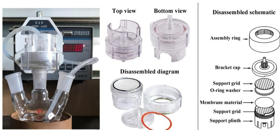
**Fig. S9** Filtration setup based on nano-adsorbent/BC composite membrane for the water treatment test.
