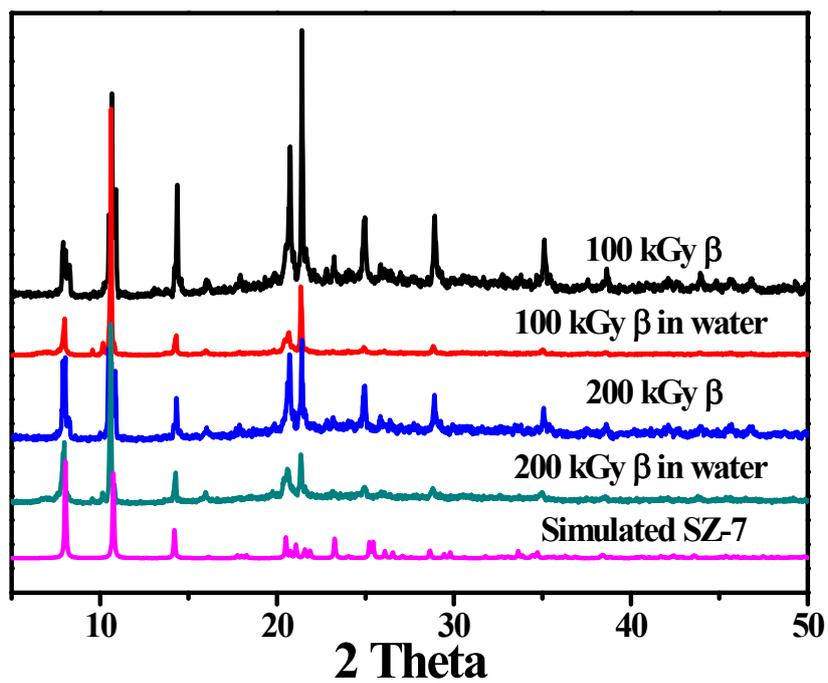
**Figure S5.** Powder X-ray diffraction patterns of SZ-7 samples after  $\beta$  radiation.
