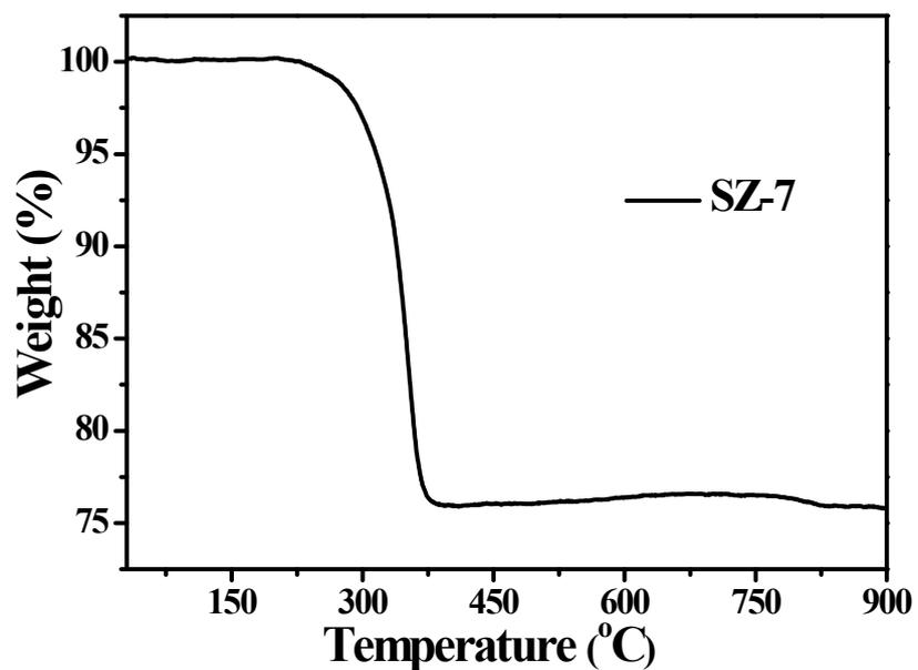
**Figure S3.** The thermogravimetric analysis data of SZ-7.
