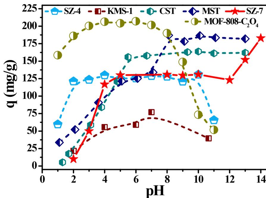
Figure S8. Comparison of the  $\text{Sr}^{2+}$  removal capacity ( $q$ ) by SZ-7 with other Sr-adsorbents at different pH values.
