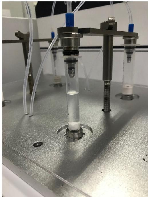
**Figure S10.** Ion-exchange column made with SZ-7 composite used in the column experiment.
