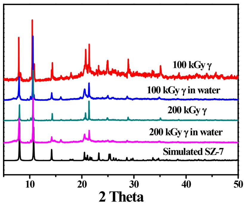
**Figure S6.** Powder X-ray diffraction patterns of SZ-7 samples after  $\gamma$  radiation.
