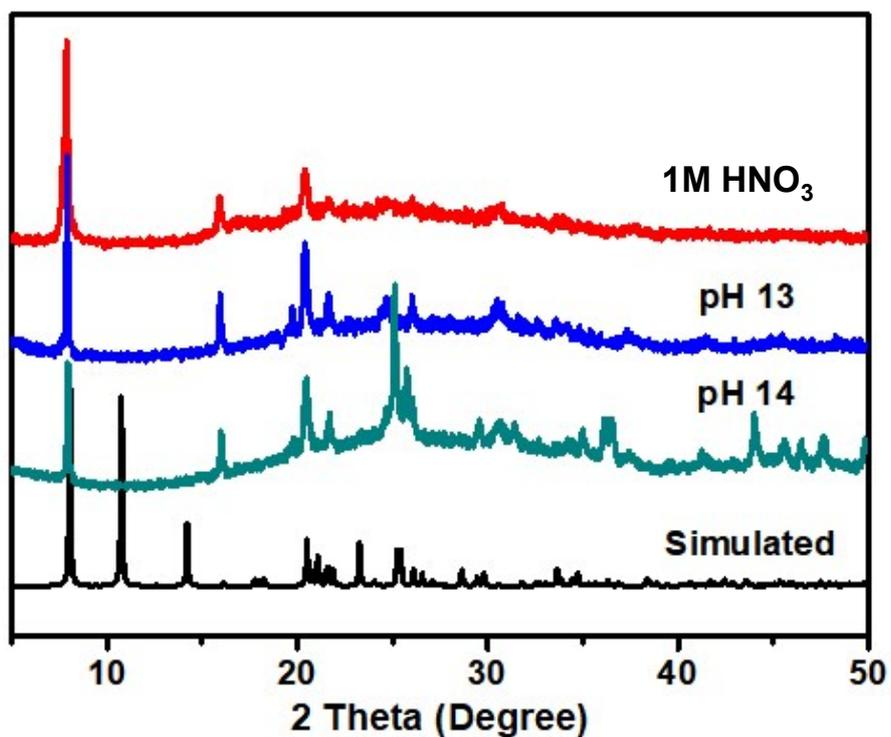
**Figure S4.** Powder X-ray diffraction patterns of SZ-7 after treatment with aqueous solutions with different pH values.
