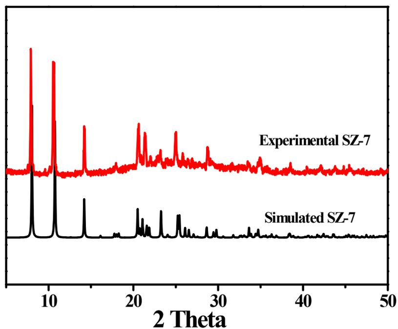
**Figure S1.** Powder X-ray diffraction patterns of SZ-7.
