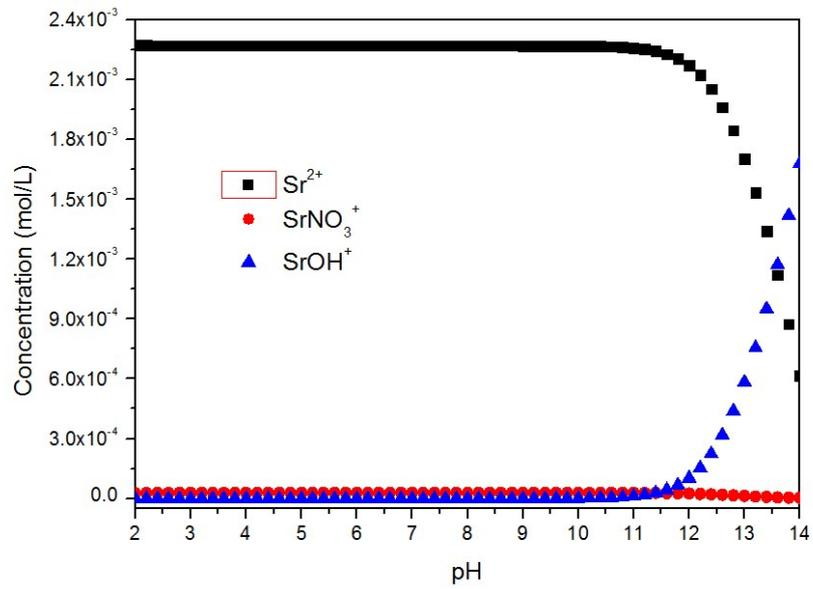
**Figure S9.** Thermodynamic calculations on the equilibrium speciation of  $\text{Sr}^{2+}$  at alkaline condition.
