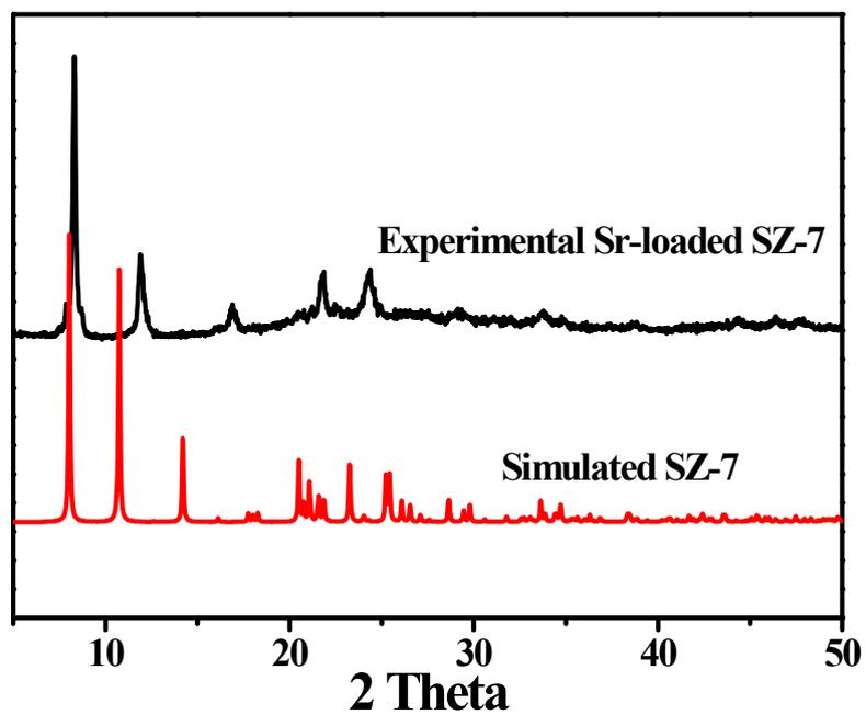
**Figure S13.** Powder X-ray diffraction patterns of experimental Sr-loaded SZ-7 samples.
