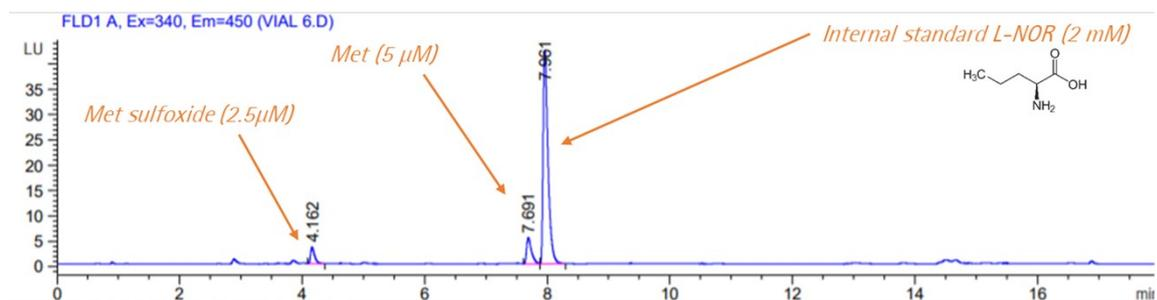
**Figure S3: chromatogram of a standard vial**
