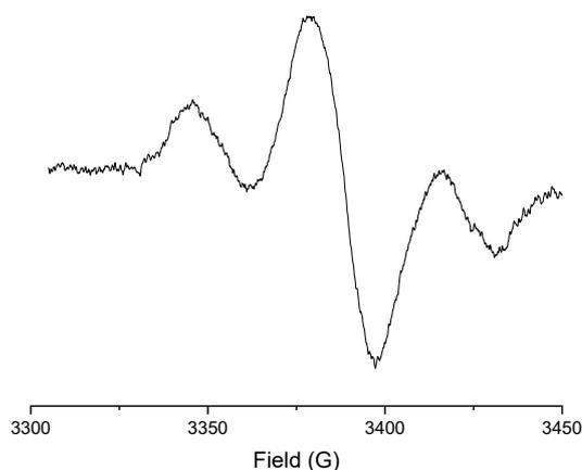
Figure S5 : ESR spectra of PE/EVOH/PE multilayer film 20 days after electron beam irradiation
