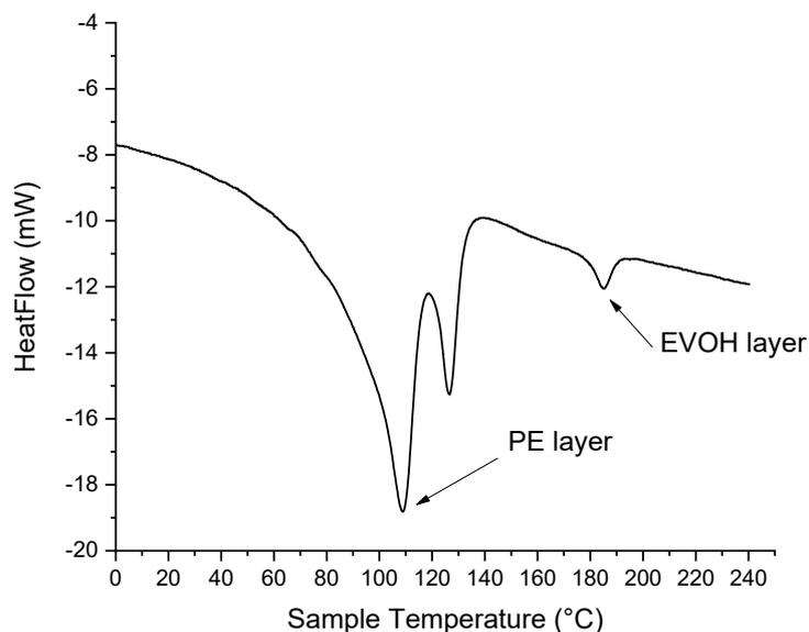
Figure S4: thermogram of electron beam irradiated sample at 50 kGy
