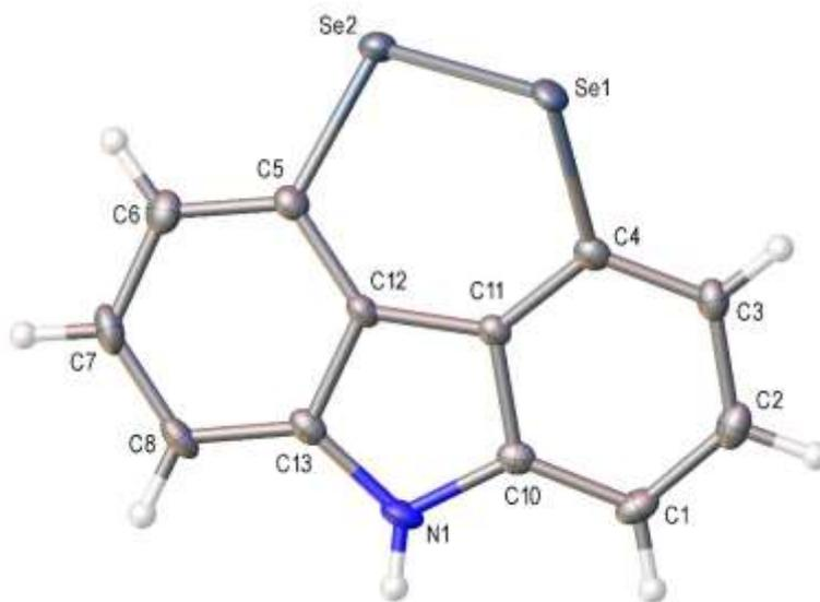
**Figure S7** Crystal structure of **12b** with ellipsoids drawn at the 50 % probability level.
