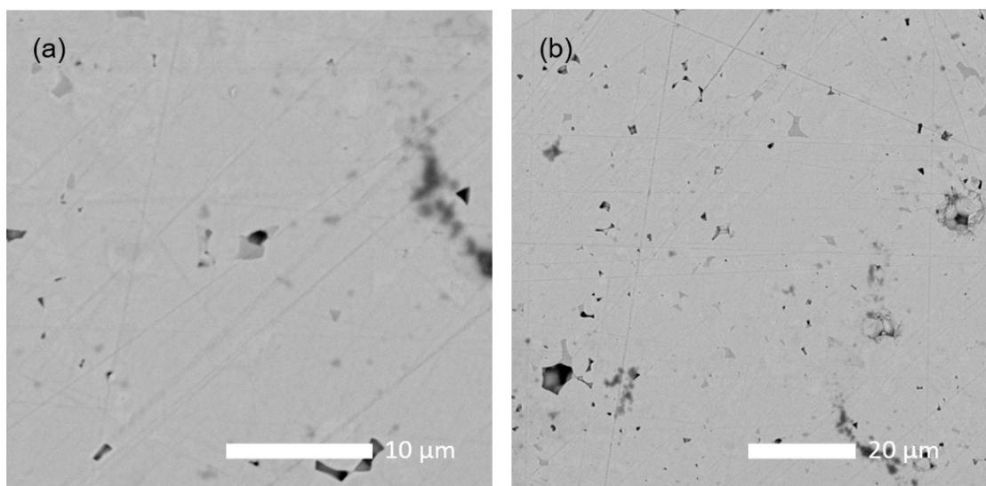
Fig S10. The surface morphology images of NA-LLZTO electrolyte membrane before the cycles.
