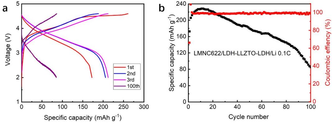
**Fig. S5.** The cyclic performance of the LMNC622/LDH-LLZTO-LDH/Li battery at 0.1C.
