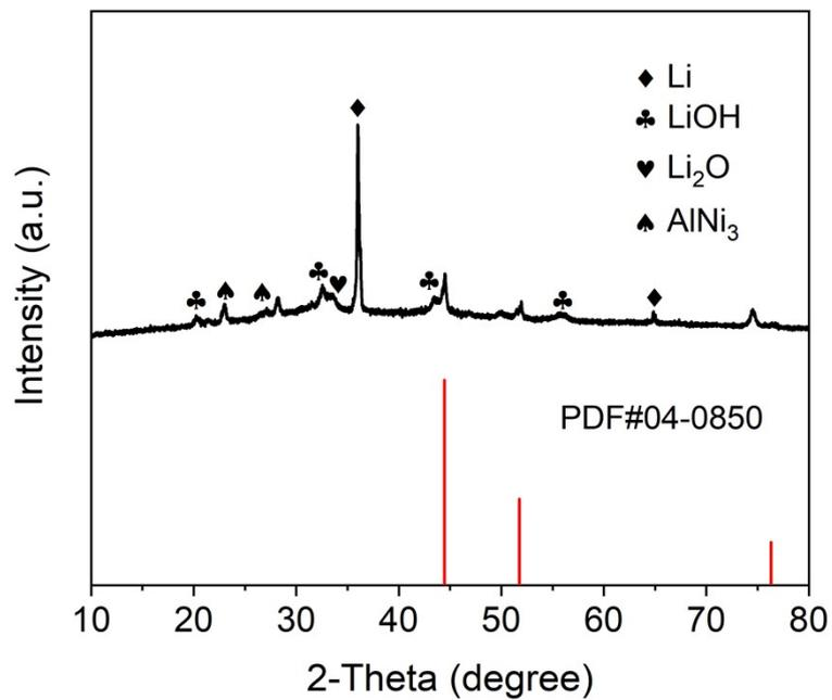
**Fig. S4.** The XRD phase of the reaction product of LDH and lithium at 300 °C.
