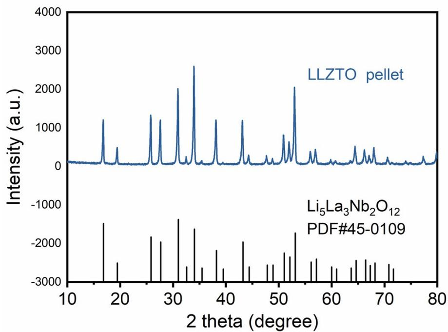
Fig. S7. The XRD of LLZTO after the alcohol.
