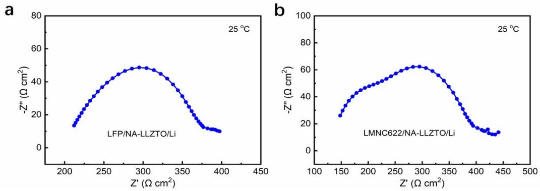
**Fig. S6.** The EIS of full battery. (a) LFP/NA-LLZTO/Li. (b) LMNC622/NA-LLZTO/Li .
