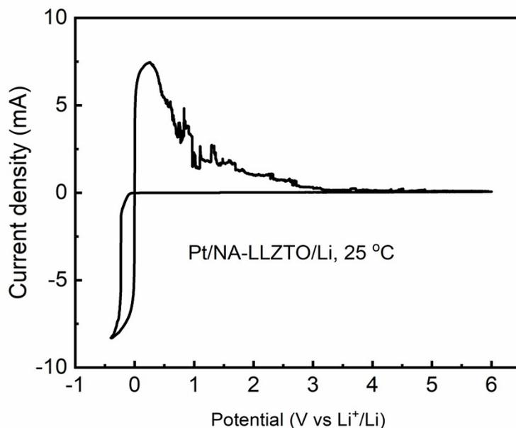
Fig S9. CV of Pt/NA-LLZTO/Li at 25 °C.
