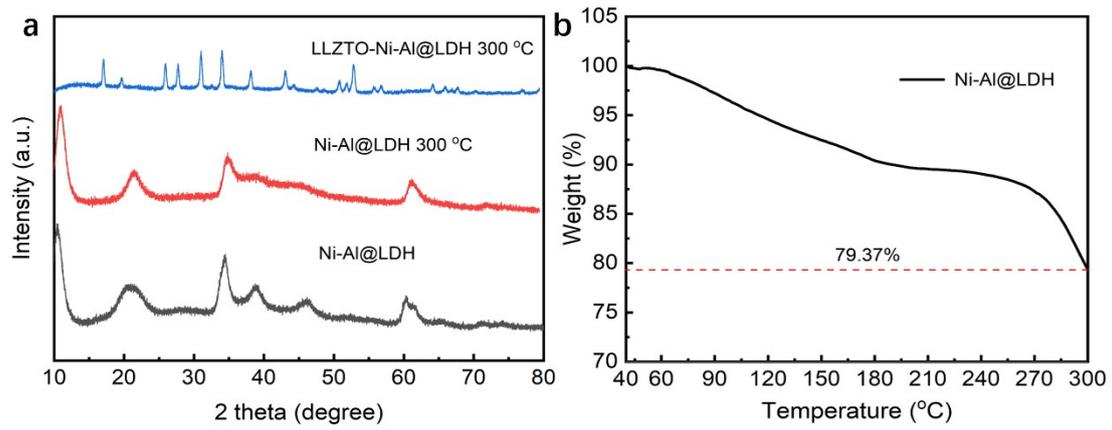
**Fig. S3.** (a) XRD of LDHs, LDHs after 300 °C heating, LDHs in LLZTO. (b) TG curve of LDHs.
