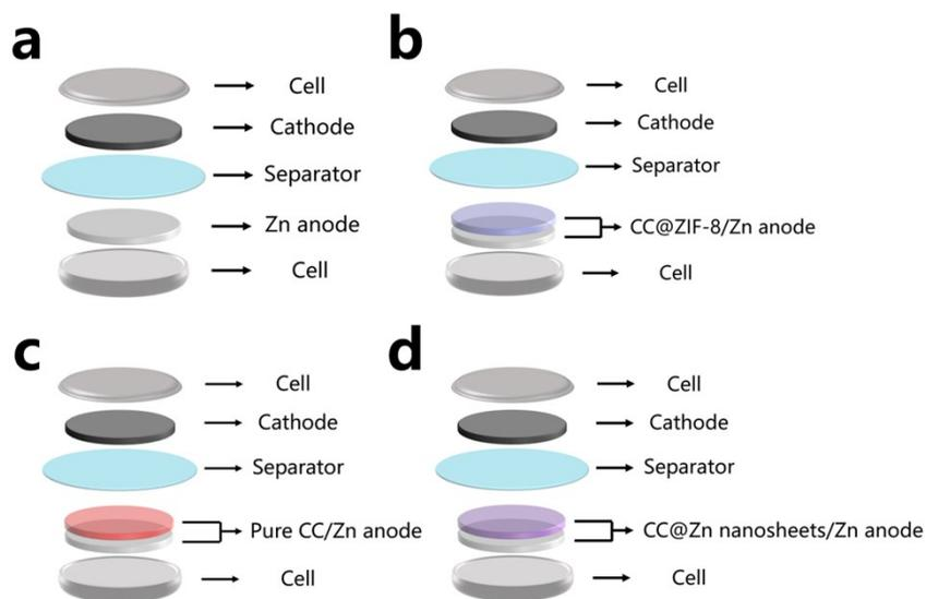
**Fig. S4.** The structural models of (a) traditional ZICs with one bare Zn anode, (b) modified ZICs with CC@ZIF-8/Zn anode, (c) pure CC/Zn anode and (d) CC@Zn nanosheets/Zn anode.
