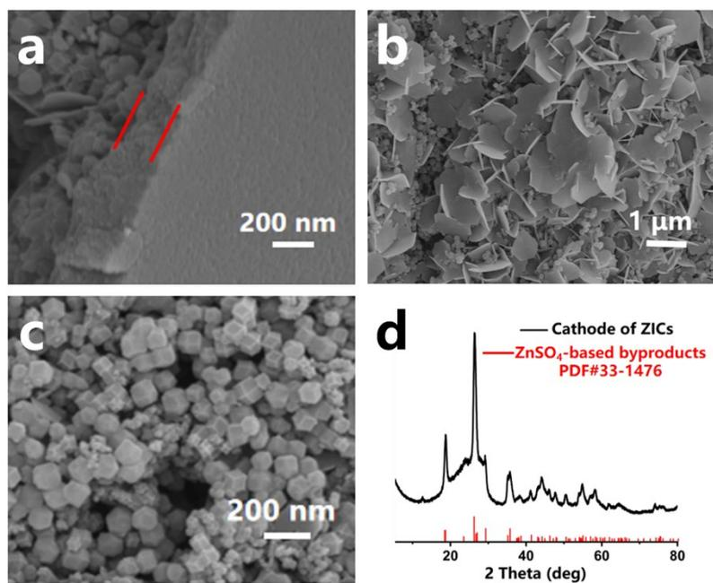
**Fig. S1.** SEM images of cathodes in different ZICs after 1000 cycles at 50 mV s<sup>-1</sup>. (a) ZIC, (b) ZIC-CC and (c) ZIC-CC/ZIF-8, respectively. XRD pattern of (d) cathode in ZIC after 1000 cycles at 50 mV s<sup>-1</sup>.
