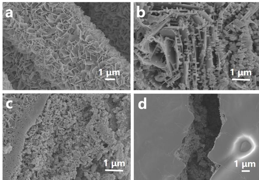
**Fig. S3.** SEM images of various components in ZIC-CC/Zn nanosheets. (a) Initial CC@Zn nanosheets, (b) CC@Zn nanosheets, (c) Zn metal anode and (d) cathode after 50 cycles at  $50 \text{ mV s}^{-1}$ .
