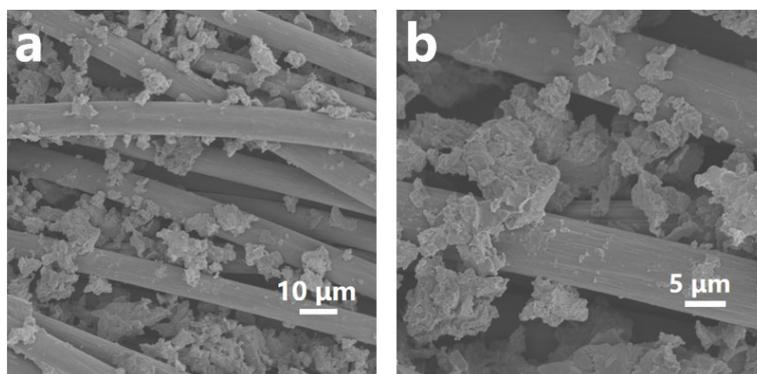
**Fig. S2.** SEM images of (a-b) large particles of Zn deposits on CC in ZIC-CC after 1000 cycles at 50 mV s<sup>-1</sup>
