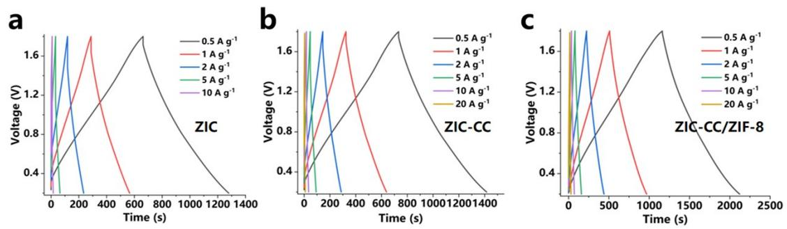
**Fig. S5.** The GCD curves of (a) ZIC, (b) ZIC-CC and (c) ZIC-CC/ZIF-8.
