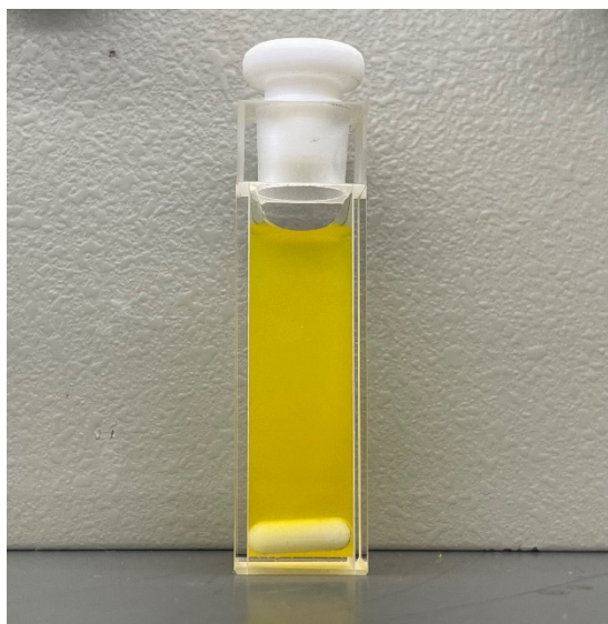
Fig. S5. Dispersion of [CO 2 H]sp 2 c-COF sample (0.5 mg/mL in buffer solution) after sonication for 5 mins.
