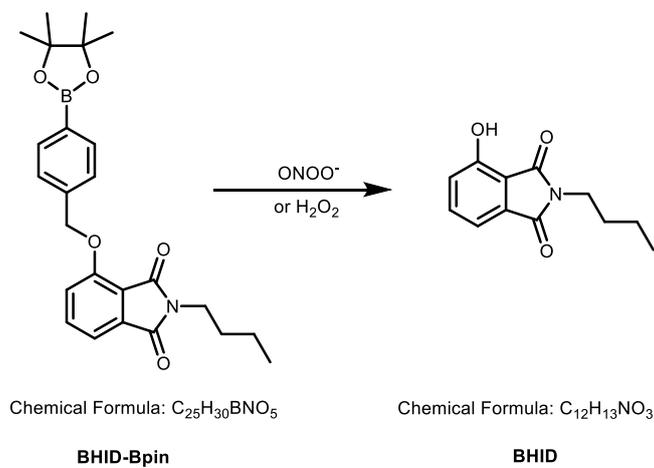
**Scheme S2.** Proposed mechanism for the reaction of probe **BHID-Bpin** upon addition of  $ONOO^-/H_2O_2$ .
