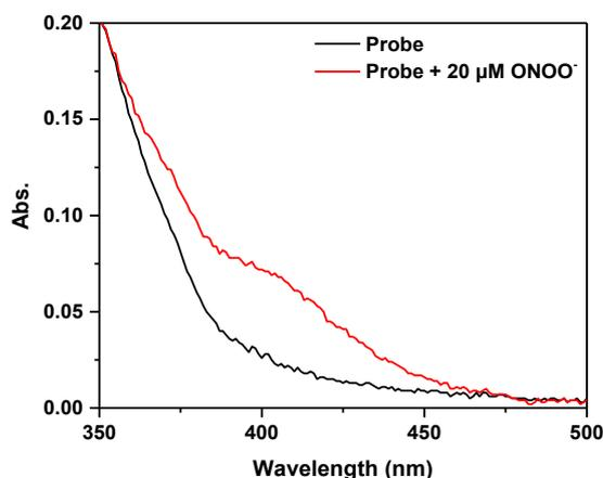
**Figure S1.** Absorption spectra of probe **BHID-Bpin** (10  $\mu$ M) with and without  $ONOO^-$  (20  $\mu$ M) in PBS buffer solution (10 mM, pH = 7.40) after 1 min.
