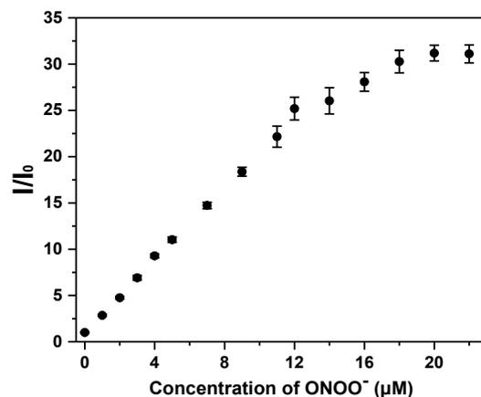
**Figure S2.** Emission at 515 nm of the probe **BHID-Bpin** (10 μM) with increasing addition of ONOO<sup>-</sup> (from 0 to 22 μM) in PBS buffer solution (10 mM, pH = 7.40) after 1 min.  $\lambda_{\text{ex}} = 400$  (bandwidth 8) nm.
