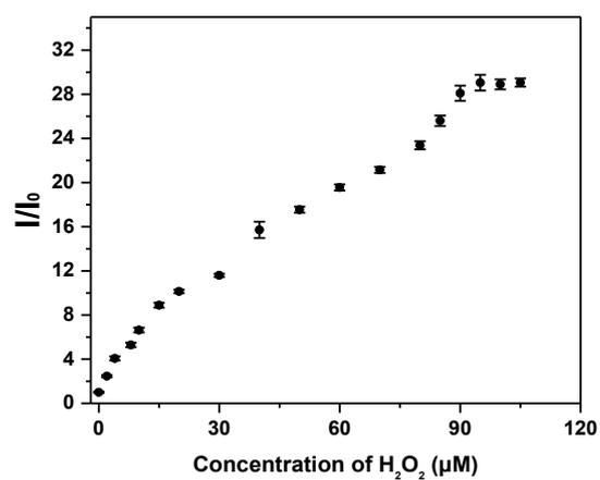
**Figure S7.** Emission at 515 nm of the probe **BHID-Bpin** (10  $\mu\text{M}$ ) with increasing addition of  $\text{H}_2\text{O}_2$  (from 0 to 105  $\mu\text{M}$ ) in PBS buffer solution (10 mM, pH = 7.40) after 80 min.  $\lambda_{\text{ex}}$  = 400 (bandwidth 8) nm.
