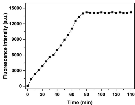
**Figure S9.** Plots of fluorescence intensity vs. the reaction time of the probe **BHID-Bpin** (10  $\mu\text{M}$ ) with 95  $\mu\text{M}$   $\text{H}_2\text{O}_2$  ( $\lambda_{\text{ex/em}} = 400$  (bandwidth 8) nm /515 nm) in PBS buffer solution (10 mM, pH = 7.40).
