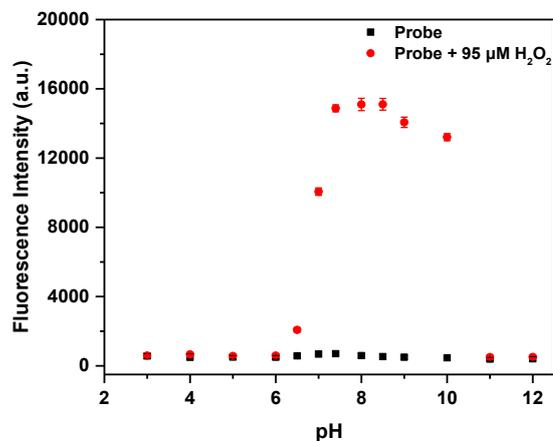
**Figure S8.** Effects of pH on the fluorescence of the probe **BHID-Bpin** (10  $\mu\text{M}$ ) in the absence and presence of 95  $\mu\text{M}$   $\text{H}_2\text{O}_2$ .  $\lambda_{\text{ex/em}} = 400$  (bandwidth 8) nm /515 nm after 80 min.
