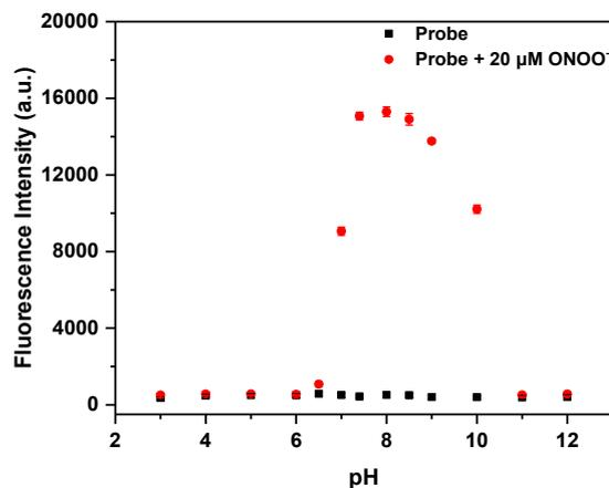
**Figure S4.** Effects of pH on the fluorescence of the probe **BHID-Bpin** (10  $\mu\text{M}$ ) in the absence and presence of  $\text{ONOO}^-$  (20  $\mu\text{M}$ ) after 1 min.  $\lambda_{\text{ex/em}} = 400$  (bandwidth 8) nm /515 nm.
