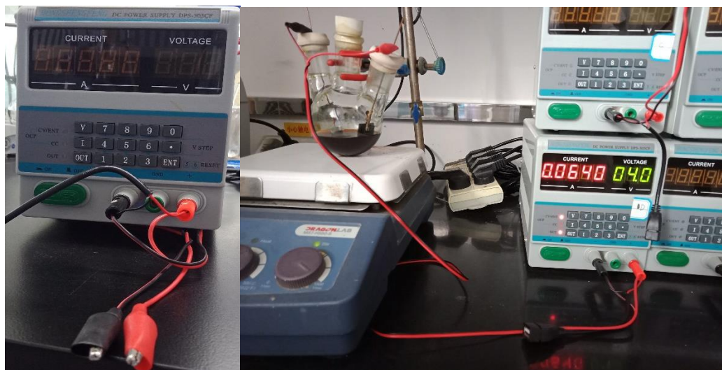
Figure S1. Instrument for electrolysis
