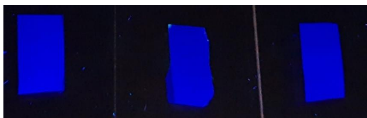
Figure S7: Photograph of compounds 3-5 (from left to right) in PMMA film (4wt%).
