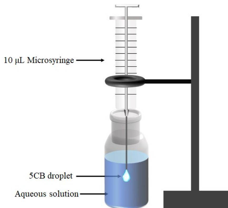
**Figure S1.** The schematic illustration of the experimental setup.
