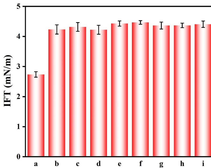
**Figure. S6.** Interfacial tensions of the pendant droplets in (a) 0.1 mM Myr, (b) TBS, and the aqueous solutions of different inhibitors: (c)  $\text{Pb}^{2+}$ , (d)  $\text{Hg}^{2+}$ , (e) DDVP, (f) dimethoate, (g) neostigmine, (h) galantamine, (i) rivastigmine.
