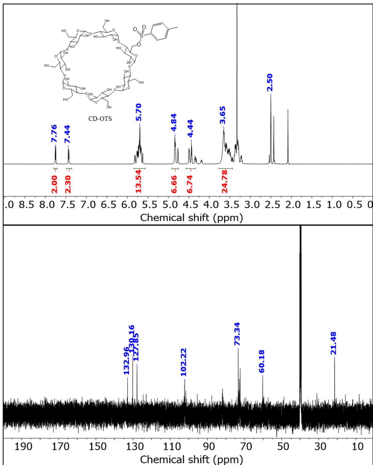
Figure S8: NMR spectra of CD-OTS
