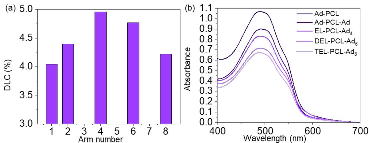
Figure S22: a) DLC values calculated for the DOX loaded CASM<sub>x</sub>; b) corresponding absorbance spectra.
