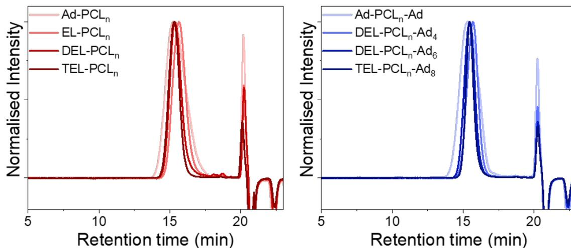
Figure S6: GPC data of all the PCL polymers measured with THF as an eluent.
