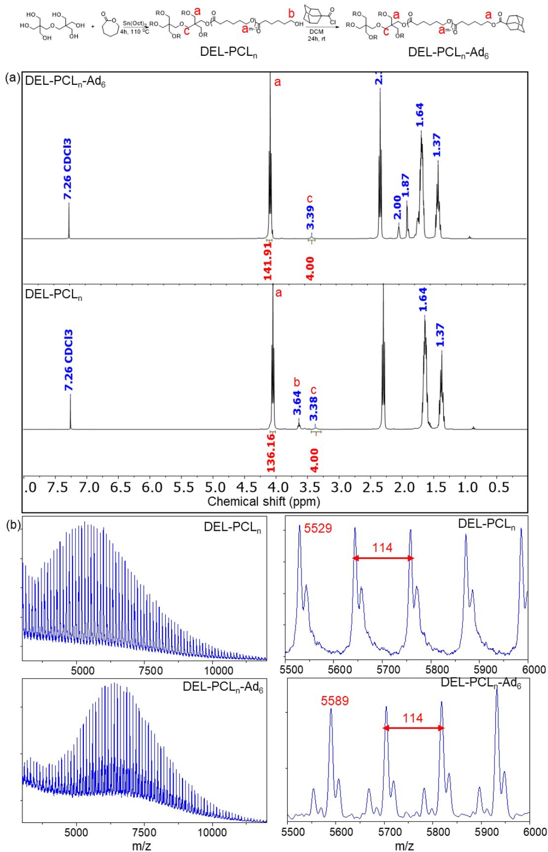
Figure S4: a) <sup>1</sup>H-NMR b) MALDI spectra of DEL-PCL<sub>n</sub> and DEL-PCL<sub>n</sub>-Ad<sub>6</sub>
