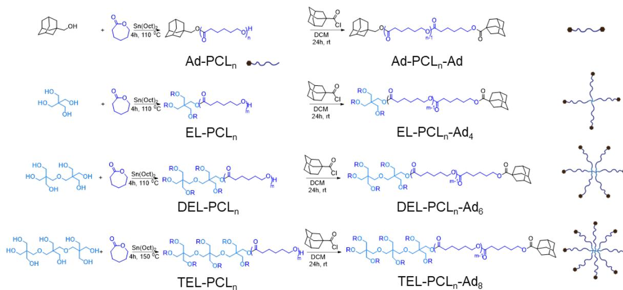
Figure S1: Synthesis scheme of different types of PCL polymers and their end group modification to give Ad terminated PCL. Cartoon representation of PCL polymers with Ad end groups is shown on the right.
