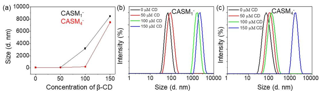
Figure S20: a) Effect of addition of  $\beta$ -CD to CASM<sub>1</sub><sup>-</sup> and CASM<sub>4</sub><sup>-</sup> and b, c) their corresponding DLS data.
