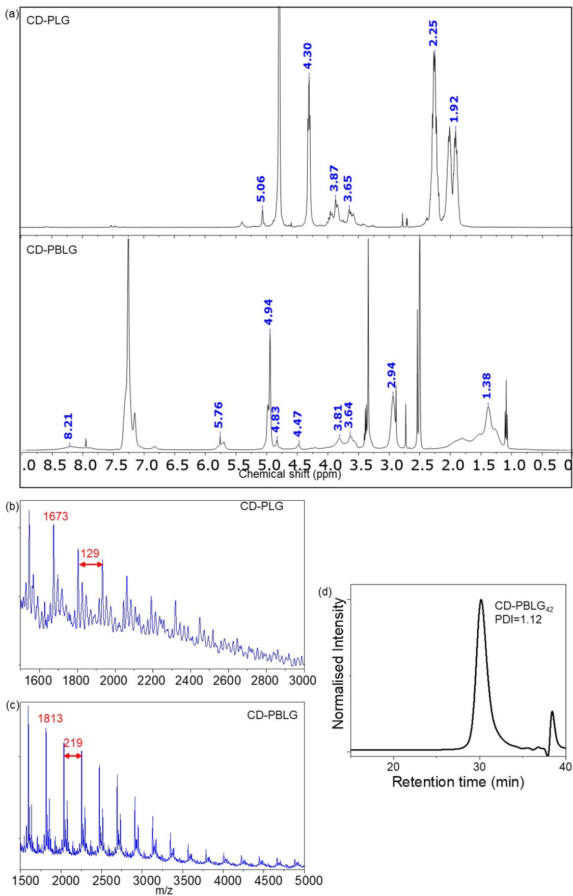
Figure S12: a)  $^1\text{H-NMR}$  of CD-PLG<sub>n</sub> (DMSO- $d_6$ ) and CD-PBLG<sub>n</sub> ( $\text{D}_2\text{O}$ ), MALDI spectra of b) CD-PLG<sub>n</sub>, c) CD-PBLG<sub>n</sub>, d) GPC chromatogram of CD-PBLG<sub>42</sub>.
