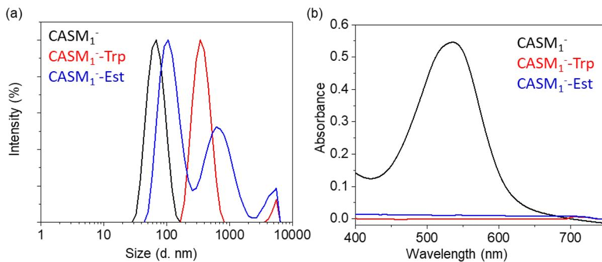
Figure S24: a) DLS data obtained for CASM<sub>1</sub><sup>-</sup> treated with esterase (Est) and trypsin (Trp). b) Absorbance spectra of Nile red loaded CASM<sub>1</sub><sup>-</sup> with and without the treatment with Est and Trp.
