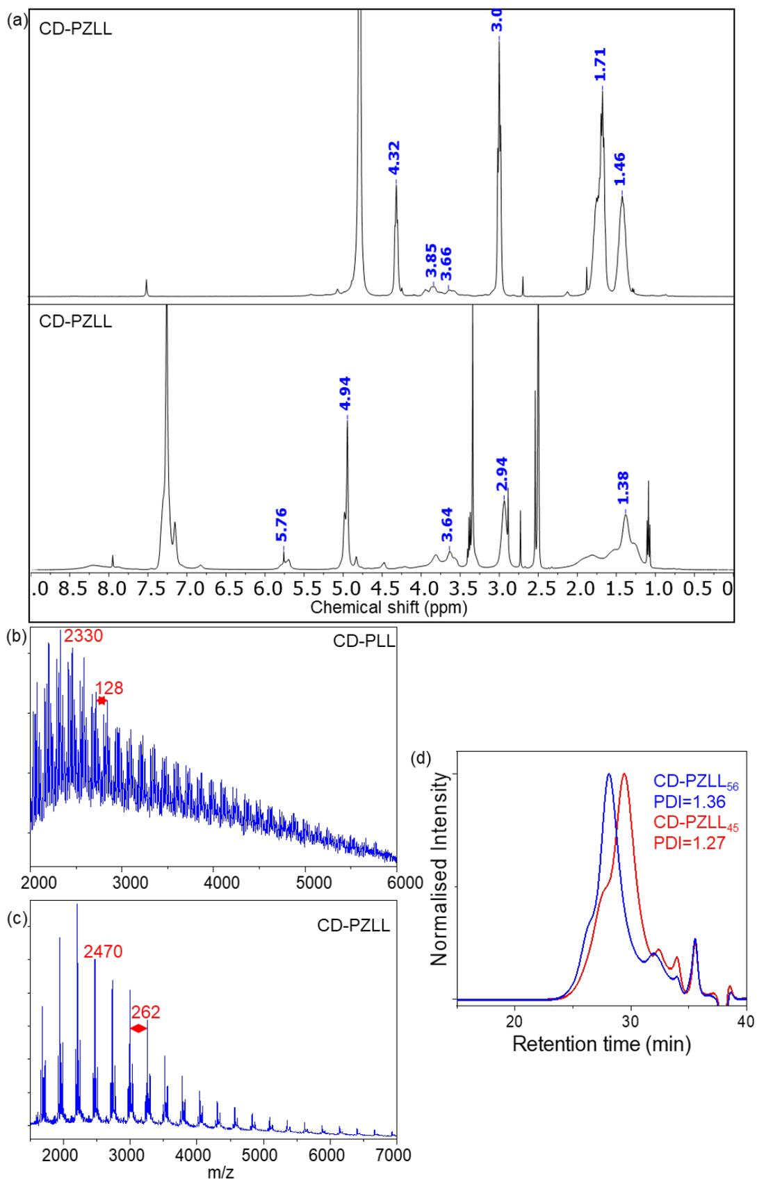
Figure S13: a)  $^1\text{H-NMR}$  of CD-PZLL<sub>n</sub>, CD-PLL<sub>n</sub>. MALDI spectra of b) CD-PLL<sub>n</sub>, c) CD-PZLL<sub>n</sub>. d) GPC data of CD-PZLL<sub>n</sub>.
