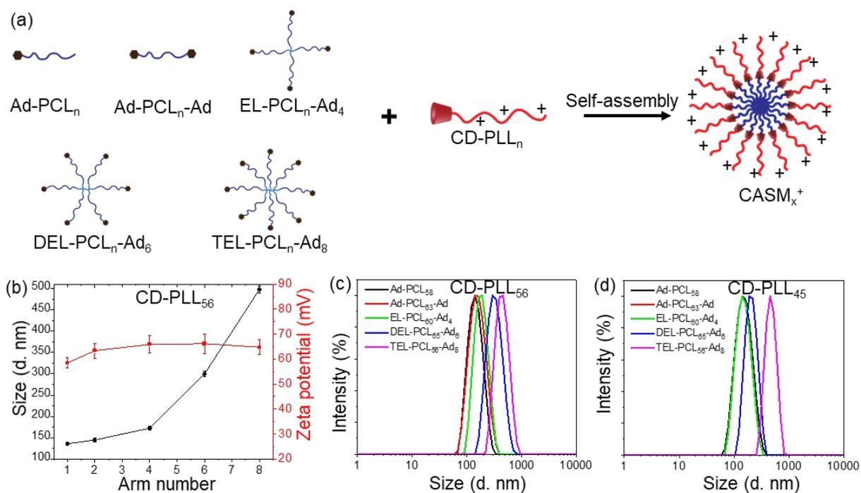
Figure S14: a) Schematic illustration of the formation of  $CASM_x^+$  from different hydrophobic components and CD-PLL. b) size and zeta potential obtained with increase in arm number. c, d) DLS data obtained for  $CASM_x^+$  with CD-PLL<sub>56</sub> and CD-PLL<sub>45</sub>.
