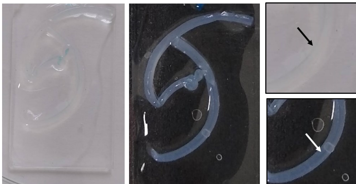
Figure S42. Photographs of filament-in-filament 2 with a white and a black background with two expanded images on the right with arrows to guide the eye to the thin blue inner filament.
