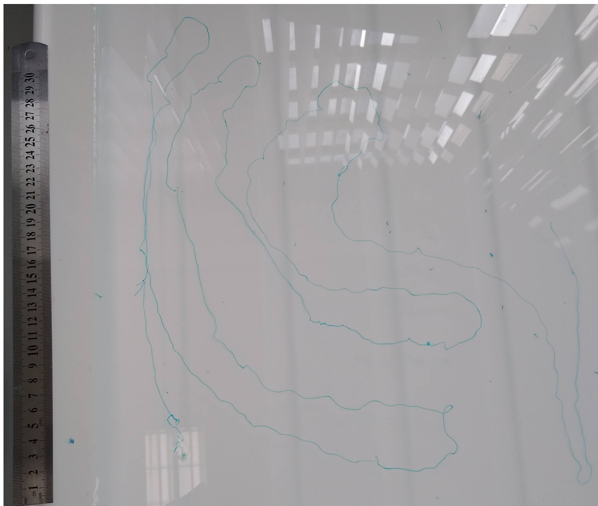
Figure S30. The full photograph of a multi-meter continuous gel filament (presented in the main paper) formed from a 10 mg/mL 1ThNapFF solution stained with 80 ppm Nile Blue A in a 50 mM \text{CaCl}_2 bath. A 30 cm ruler is placed to the left of the photograph for scale.
