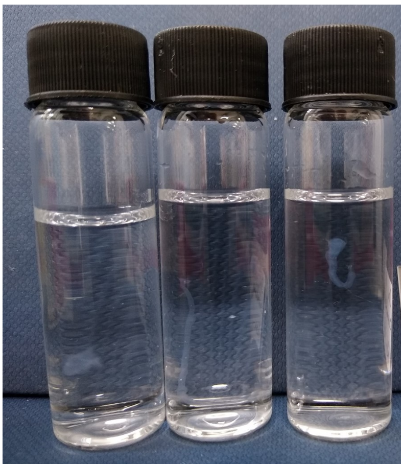
Figure S18. Photograph of gel filaments formed using a 20-200 \mu\text{L} pipette at slow (left), intermediate (middle) and fast (right) injection speeds
