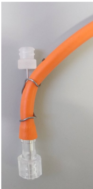
Figure S3. Photograph showing the alignment of a needle within the rubber tubing and Luer-lock nozzle for the sheath flow. Note the metal wire is shaped to manipulate the rubber tubing to aid with this.
