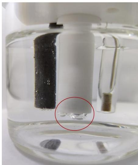
**Fig. S11.** The electrochemical device of HzOR for  $\text{Co}_6\text{W}_6\text{C}@\text{C}$ .
