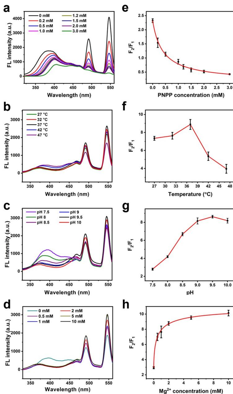
**Figure S6.** The left column: the effect of (a) PNPP concentration, (b) temperature, (c) pH, (d)  $Mg^{2+}$  concentration to the fluorescence spectra of  $g-C_3N_4:Tb$ -PEG NSs ( $100 \mu g mL^{-1}$ ). The right column: the effect of (e) PNPP concentration, (f) temperature, (g) pH, (h)  $Mg^{2+}$  concentration to the ratiometric fluorescence response of the probing system based on IFE.
