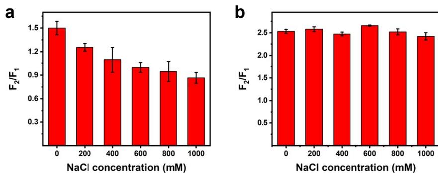
**Figure S3.** The variation of ratiometric fluorescence responses of 100  $\mu\text{g mL}^{-1}$  (a) g- $\text{C}_3\text{N}_4:\text{Tb}$  nanosheets and (b) g- $\text{C}_3\text{N}_4:\text{Tb-PEG}$  nanosheets with various concentrations of NaCl in the range of 0-1000 mM.
