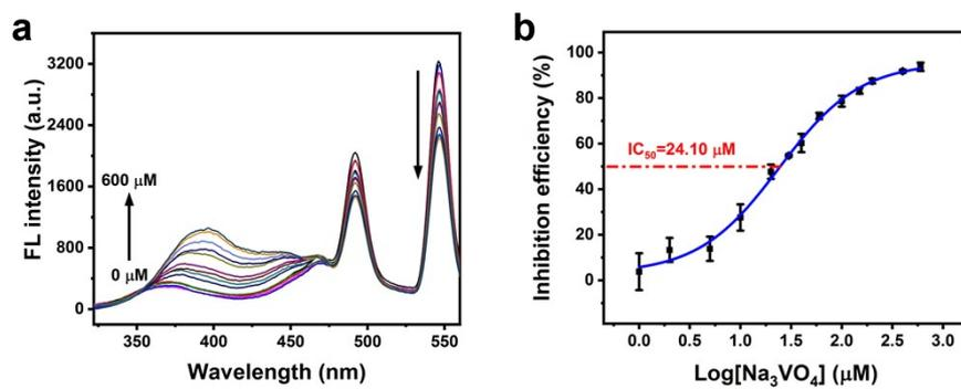
**Figure S8.** (a) Fluorescence responses of g- $\text{C}_3\text{N}_4$ :Tb-PEG nanosheets in the presence of various concentration of  $\text{Na}_3\text{VO}_4$  (0-600  $\mu\text{M}$ ). (b) Inhibition efficiency as a function of the logarithmic concentration of  $\text{Na}_3\text{VO}_4$ .
