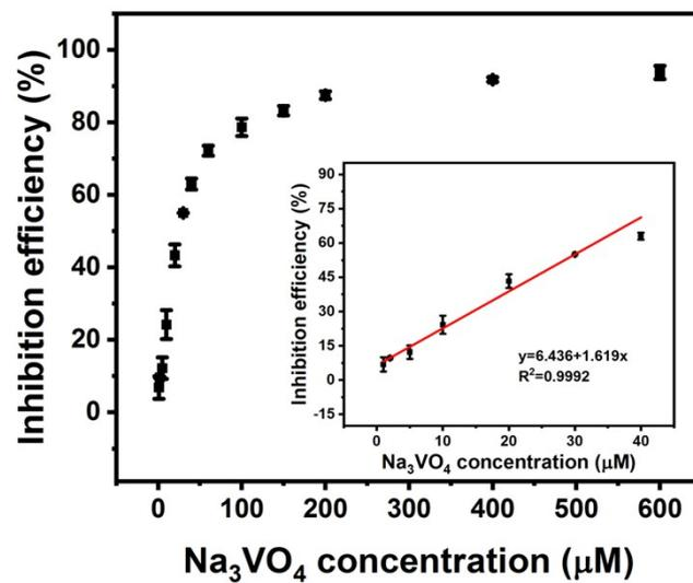
**Figure S9.** Fluorescence responses of g- $\text{C}_3\text{N}_4$ :Tb-PEG NSs in the presence of various concentration of  $\text{Na}_3\text{VO}_4$  (0-600  $\mu\text{M}$ ). Inset: the linear relationship between the inhibition efficiency and  $\text{Na}_3\text{VO}_4$  concentration in the range of 1-40  $\mu\text{M}$ .
