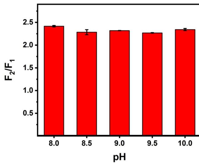
**Figure S4.** The ratiometric fluorescence response of  $g\text{-C}_3\text{N}_4\text{:Tb-PEG NSs}$  ( $100 \mu\text{g mL}^{-1}$ ) under different pHs.
