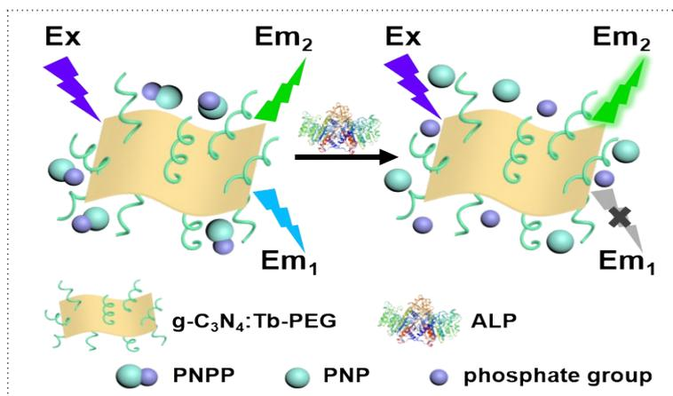
**Scheme S1.** The illustration for the ratiometric fluorescence strategy with g-C<sub>3</sub>N<sub>4</sub>:Tb-PEG nanosheets as the probe for the detection of ALP activity based on inner filter effect.
