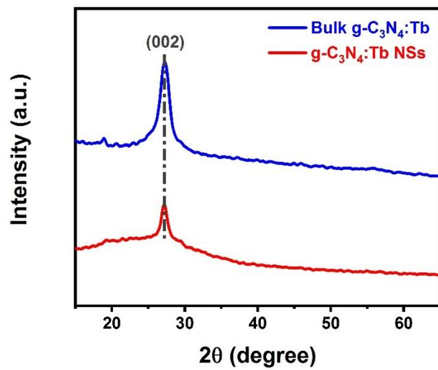
**Figure S1.** XRD patterns of the bulk g-C<sub>3</sub>N<sub>4</sub>:Tb and the g-C<sub>3</sub>N<sub>4</sub>:Tb NSs after ultrasonic treatment.
