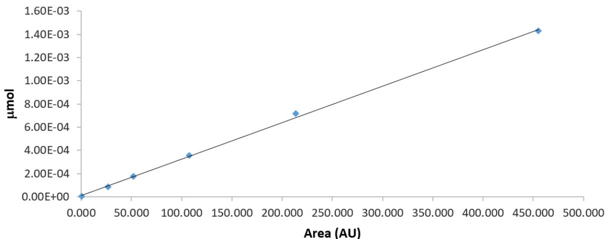
**Figure S2.** Calibration curve of **1a** for the determination of the molar activity
