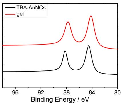
**Figure S5.** XPS results exhibiting the binding energy of Au(4f) of TBA-AuNCs and
