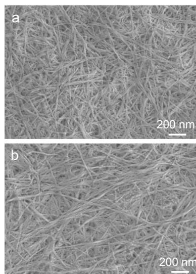
**Figure S14.** SEM image of (a) S-MA/AuNCs gel and (b) R-MA/ TBA-AuNCs gel at  $c_{MA} = 30$  mM.
