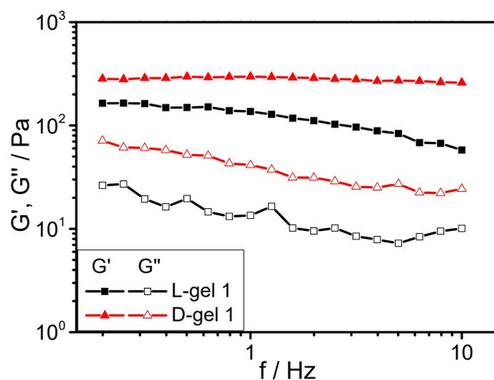
**Figure S7.** Rheological profiles ( $G'$  and  $G''$  as a function of frequency ( $\tau=1 \text{ Pa}$ ) of L-gel 1 and D-gel 1.
