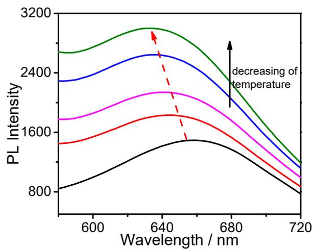
**Figure S4.** Temperature-dependent PL spectra of **L-gel 1**.
