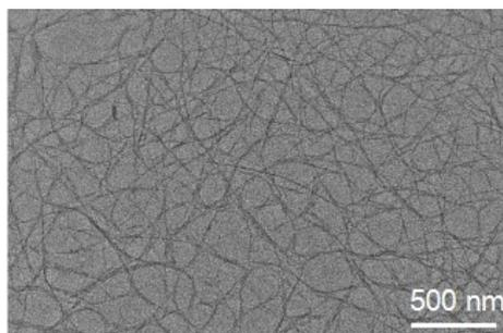
**Figure S6.** TEM image of the TBA-AuNCs ( $c_{\text{HAuCl}_4}=5 \text{ mg mL}^{-1}$ ).
