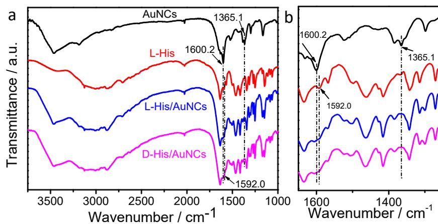
**Figure S9.** FT-IR spectra of TBA-AuNCs, L-His and L/D-His/ TBA-AuNCs. (a is the entire spectra, b is the amplifying partial spectra)
