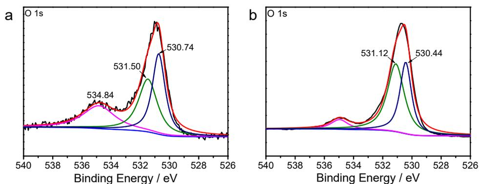
**Figure S11.** High resolution XPS spectra for O 1s of (a) TBA-AuNCs and (b) L-gel 1.
