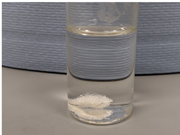
Figure S4. Image of the colourless crystals produced from the hydrothermal synthesis of \text{Ca}(\text{FU})(\text{H}_2\text{O})_3 .
