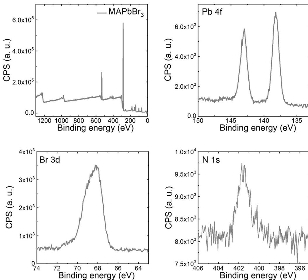
**Figure S5.** X-ray photoelectron spectra of the purified MAPbBr<sub>3</sub> PNC powders. High-resolution XPS analyses further confirmed the elemental composition of PNCs: lead (4f) at 138.2 and 143.1 eV, nitrogen (1s) at 401.9 eV, and bromine (3d) at 68.3 eV.
