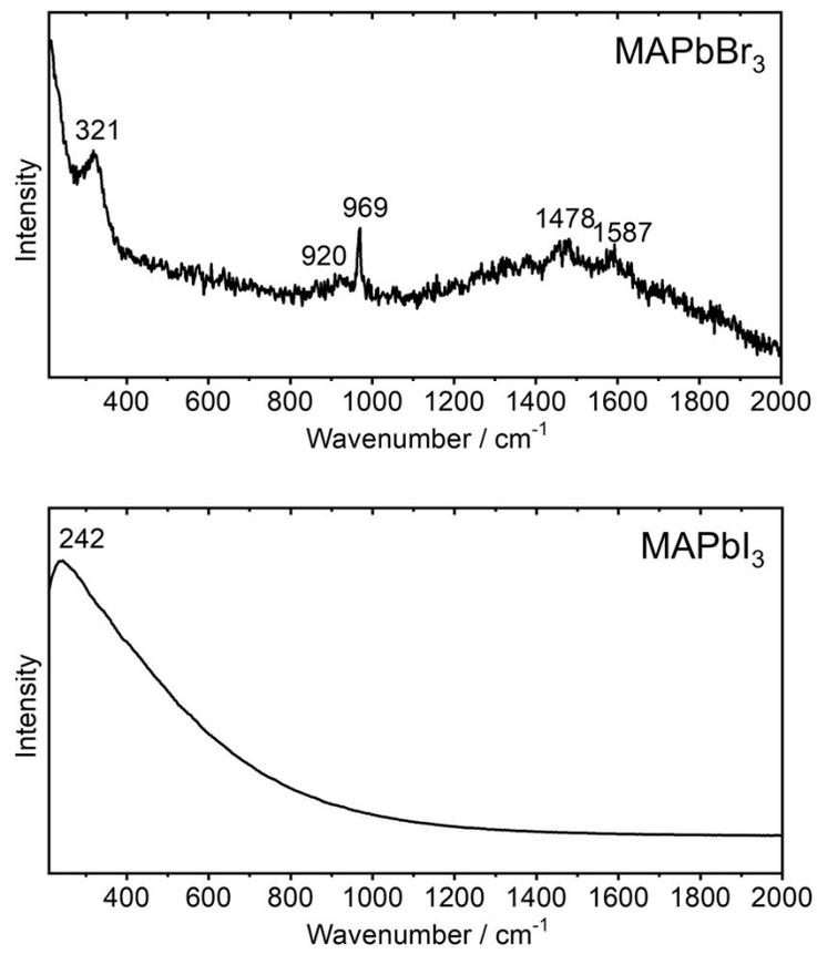
**Figure S4.** Raman spectra of MAPbBr<sub>3</sub> and MAPbI<sub>3</sub> PNC powders measured at room temperature under ambient conditions (excitation wavelength: 784.9 nm).
