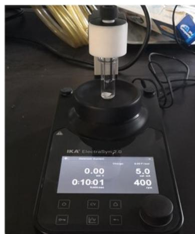
**Figure S1.** Instrumental setup of the EC synthesis of PNCs. (a) Image of the general components including the electrolysis cell graphite electrode, and the metal foils. (b) The overall setup of IKA® ElectroSyn 2.0 package for the synthesis of PNCs.
