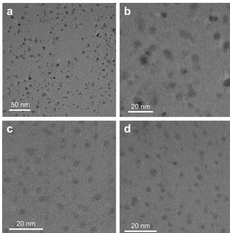
**Figure S2.** Additional bright-field TEM images of (a, b) MAPbBr<sub>3</sub> and (c, d) MAPbI<sub>3</sub> PNCs.
