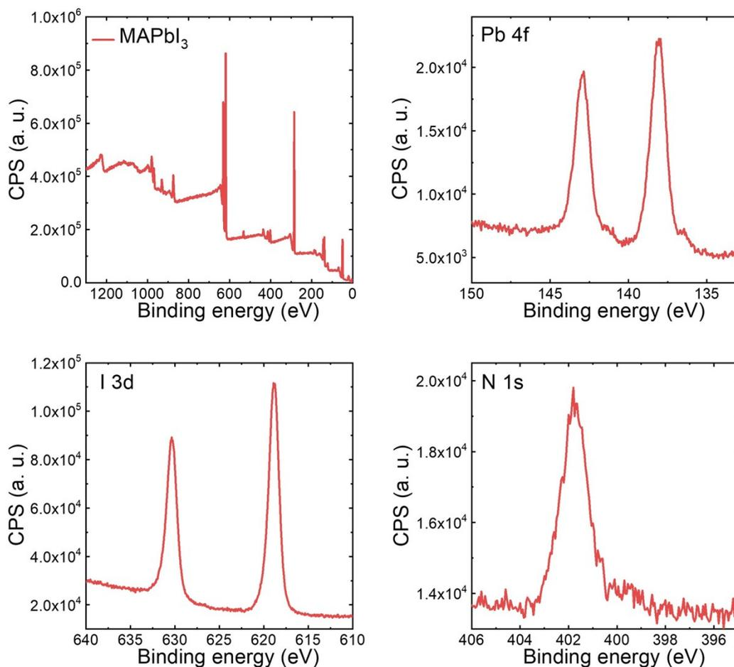
**Figure S6.** X-ray photoelectron spectra of the purified MAPbI<sub>3</sub> PNC powders. High-resolution XPS analyses further confirmed the elemental composition of PNCs: lead (4f) at 138.2 and 143.1 eV, nitrogen (1s) at 401.9 eV, and iodine (3d) at 618.8 and 630.4 eV.
