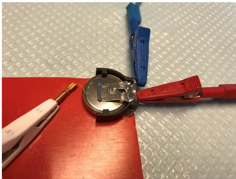
Fig. S1 Photograph of the cell '3-e E/S=7 LiAu' as an example of the three-electrode cell setup. The polyimide-wrapped Au microwire can be observed on the left. Polyimide coating on the last 5 mm of the outer end of the wire was scraped off, and then clamped by a pair of a pin and a socket of the D-miniature electrical connector, which is held by the white crocodile clip.
