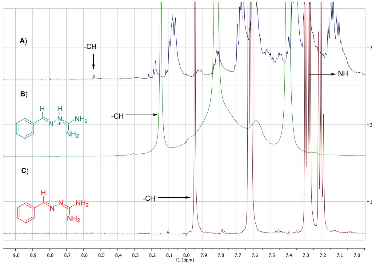
**Figure S5:** Expanded  $^1\text{H}$  NMR spectrum of C1 and its protonated form (For clear visibility of – CH peak).
