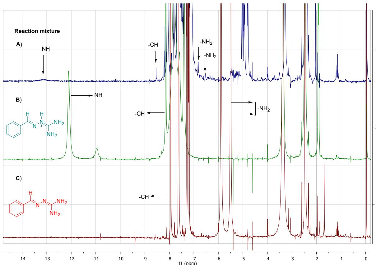
**Figure S3:** Overlapped <sup>1</sup>H NMR Spectrum A) Reaction mixture, B) Protonated azine (**C6**), C) 1,1-diaminoazine (**C1**).
