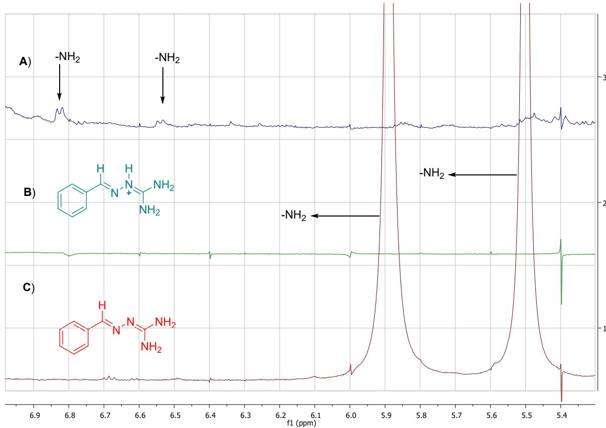
**Figure S6:** Expanded  $^1\text{H}$  NMR spectrum of C1 and its protonated form (For clear visibility of –NH<sub>2</sub> peaks).
