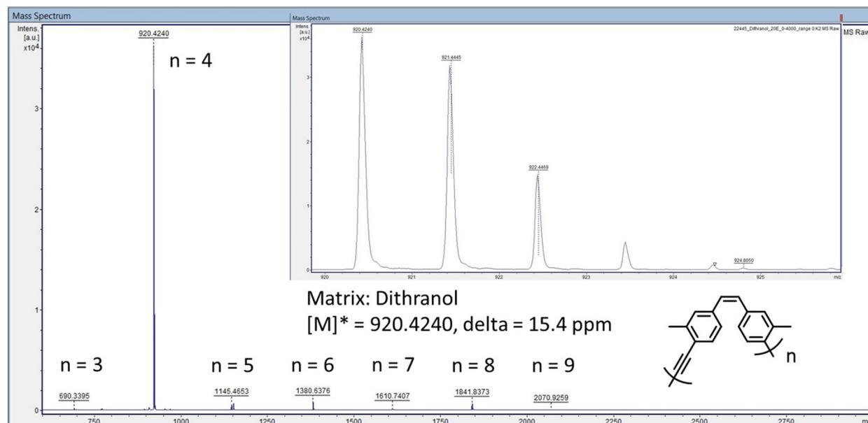
**Figure S11.** MALDI spectra of the macrocyclic products after alkyne metathesis.
