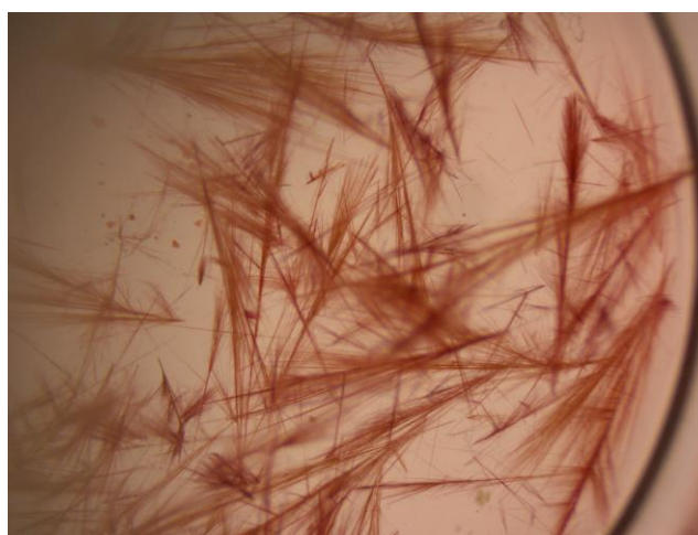
Figure S4. Crystal photos of compound 1 . Needle-like single crystals were obtained for 1 upon vapour diffusion of ethyl ether into the chloroform solution. Unfortunately, we failed to get the X-ray structures since these crystals were unstable under the desolvation conditions.
