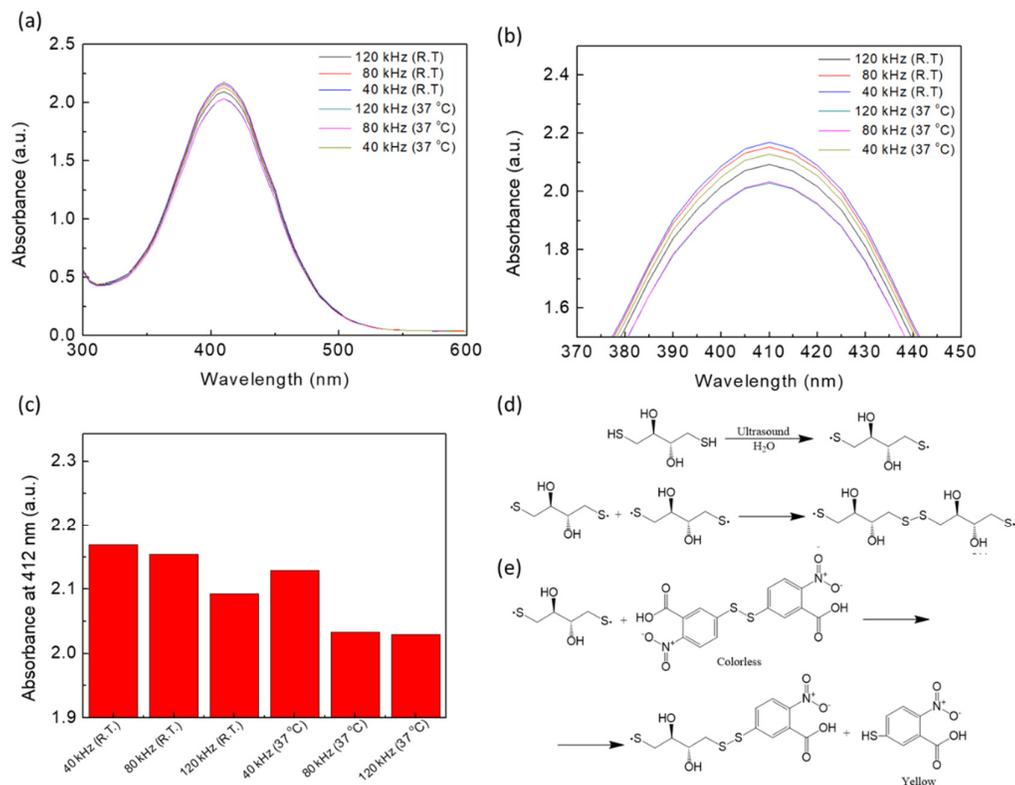
**Fig. S7** Measurements of free thiols in the solution using Ellman's assay. (a, b) Absorption spectra and (c) absorbance at 412 nm of the solutions of DTT (10 mM), KPS (0.617 M), and DTNB (2 mM) mixtures under ultrasound irradiation at different frequencies and temperatures. Schematic illustrations of (d) disulfide bond formation between DTT molecules under ultrasound irradiation and (e) reaction of thiolate radicals with DTNB.
