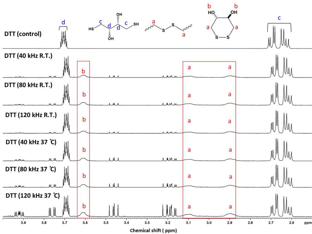
**Fig. S9** NMR spectra of DTT molecules after the ultrasound treatments in the presence of KPS (1 wt%) under different frequencies at room temperature or 37 °C.
