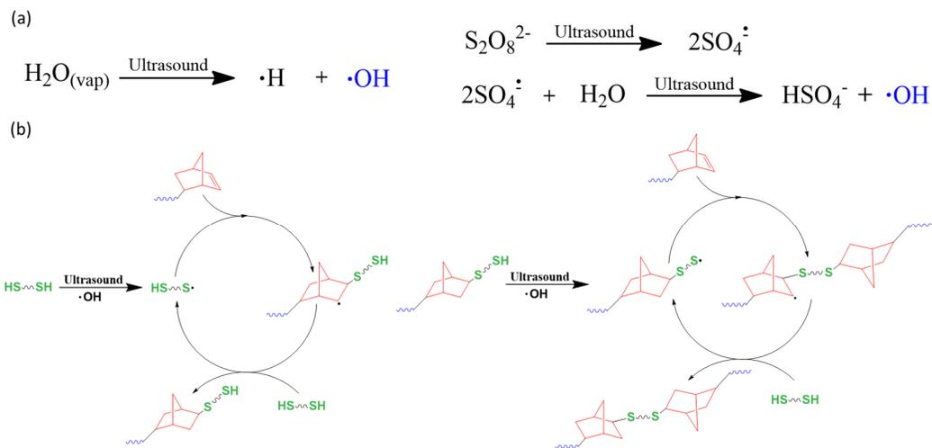
**Scheme S1.** (a) Radicals generated from water vapor and KPS under ultrasound. (b) Nor-Dex hydrogel formation through the ultrasound-initiated thiol-norbornene reaction between Nor-Dex and DTT.
