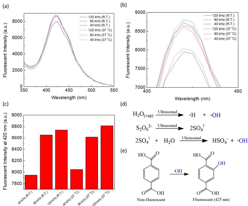
**Fig. S6** Measurements of radical amounts in the solution. (a, b) Fluorescence spectra and (c) fluorescent intensity at 420 nm of the solutions of terephthalic acid and KPS mixtures under ultrasound irradiation at different frequencies and temperatures. Schematic illustrations of (d) radical formation under ultrasound irradiation and (e) reaction of hydroxyl radical ( $\cdot\text{OH}$ ) with terephthalic acid.
