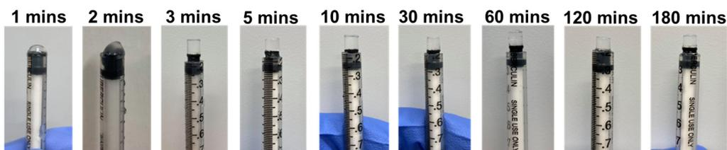
**Fig. S3** Representative images of Nor-Dex hydrogels prepared with varied sonication times (Nor-Dex (10 wt%), DTT (thiol/norbornene ratio  $N=1$ ), KPS (1.5 wt%), and 120 kHz at R.T.).
