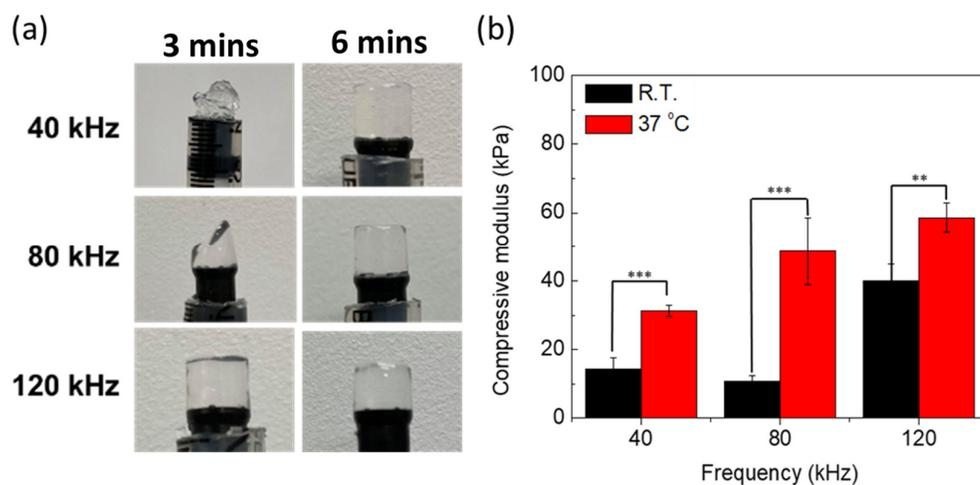
**Fig. S5** (a) Representative images of Nor-Dex hydrogels prepared in the absence of KPS at different frequencies with varied sonication times (Nor-Dex (10 wt%), DTT ( $N= 1$ )). (b) Compressive moduli of Nor-Dex hydrogels prepared in the absence of KPS with varied frequencies and temperatures (Nor-Dex (10 wt%), DTT ( $N= 1$ ), and sonication time of 6 mins). Significance was set at  $p < 0.05$  with \*\* or \*\*\* indicating  $p < 0.01$  or 0.001, respectively.
