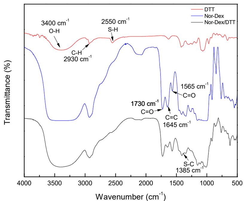
**Fig. S2** FTIR spectra of DTT, Nor-Dex polymer, and Nor-Dex hydrogel crosslinked with DTT (Nor-Dex/DTT). Nor-Dex hydrogel was prepared using Nor-Dex (10 wt%), DTT (thiol/norbornene ratio  $N=1$ ), KPS (1.5 wt%), and 120 kHz for 3 mins at R.T.
