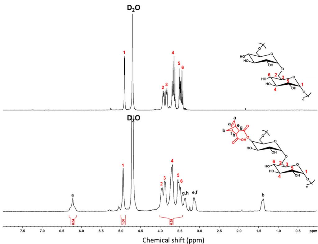
**Fig. S1**  $^1\text{H}$  NMR spectra of dextran and Nor-Dex.
