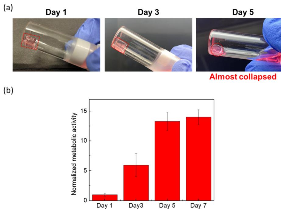
**Fig. S10** (a) Stability test of Nor-Dex hydrogel in cell culture media. (b) Normalized metabolic activity of MEFs incubated with the cell culture media including the degradation products of the Nor-Dex hydrogels.
