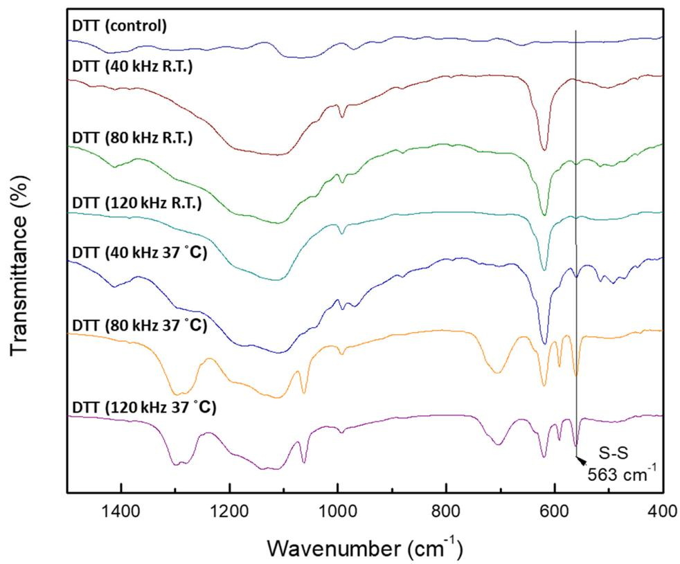
**Fig. S8** FTIR spectra of DTT molecules after the ultrasound treatments in the presence of KPS (1 wt%) under different frequencies at room temperature or 37 °C.
