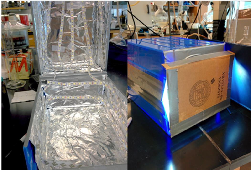
**Figure S2.** Experimental set-up for irradiation of **1-SP/MCH<sup>+</sup>** samples. A strand of broad-spectrum white LED lights taped along the foil-lined top and sides of two polypropylene bins duct-taped together with a foil-lined cardboard opening. A small hot-plate/oil bath was placed inside for temperature-controlled experiments.
