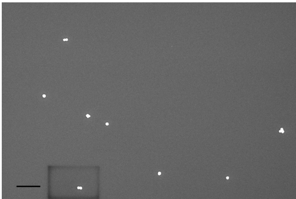
Figure S9. SEM image of the gold-coated zero-valent iron core-iron oxide shell magnetic nanoparticles. scale bar 1 \mu\text{m} .
