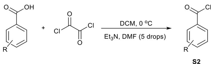
To a suspension of benzoic acid (20 mmol, 1.0 equiv) in DCM (20 mL), oxalyl chloride (5.1 g, 40 mmol, 2.0 equiv) was added dropwise at 0 °C. After that five drop of DMF was added, and stirred at room temperature until the acid was completely consumed (monitored by TLC). The solvent and excess oxalyl chloride were removed by vacuum and the residual benzoyl chloride derivative **S2** was directly used in the following step.
