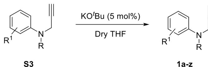
An oven dried 50 mL flask was equipped with a magnetic stir bar and compounds **S3** ( 5.0 mmol, 1.0 equiv) in dry THF (10 mL), then  $KO^tBu$  (28 mg, 0.25 mmol, 0.05 equiv) was added at 0 °C. The reaction mixture was then allowed to come to the room temperature and stirred for 0.5-1.0 h (monitored by TLC). The solvent was removed under reduced pressure. The residue was purified by column chromatography on silica gel (hexane/ethyl acetate) to give the allenamide **1a-z** (80-90%).
