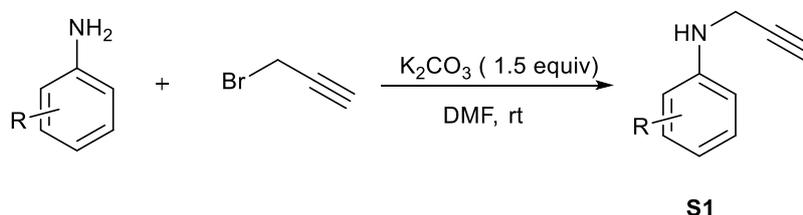
To a solution of aniline (20.0 mmol, 1.0 equiv) in DMF (30.0 mL), 3-bromopropyne (2.4 g, 20.0 mmol, 1.0 equiv) and potassium carbonate (4.2 g, 30.0 mmol, 1.5 equiv) were added. Then the mixture was stirred for 12 h at room temperature. The solution was diluted with DCM (20 mL) and washed with aqueous HCl (4 M, 2 × 30 mL), and brine solution (30 mL). The organic layer was separated, dried over  $Na_2SO_4$ , and the solvent was removed in vacuo. *N*-(prop-2-yn-
