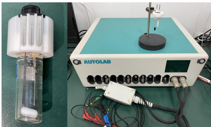
Figure S2. Pictures of Autolab83943 potentiostat. for Cyclic voltammograms
