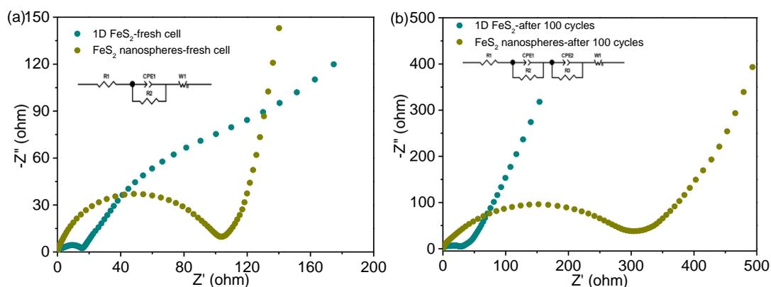
**Fig. S11** EIS spectra of CWE FeS<sub>2</sub> and the FeS<sub>2</sub> nanospheres (a) before and (b) after cycling 100 times at 1 A g<sup>-1</sup>. The inserts display the equivalent circuit models.
