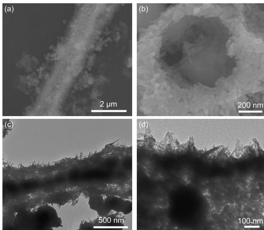
**Fig. S3** (a,b) SEM and (c,d) TEM images of CWE FeS<sub>2</sub>.
