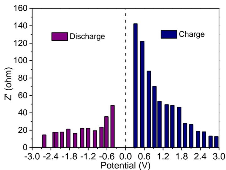
**Fig. S10** The charge transfer resistance within one charge-discharge cycle.
