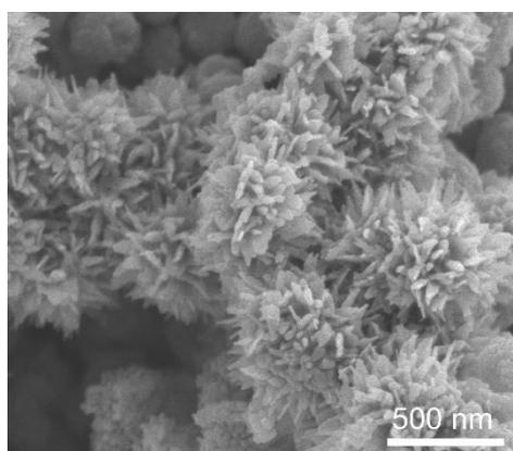
**Fig. S4** SEM image of the yolk-shell FeS<sub>2</sub> nanospheres.
