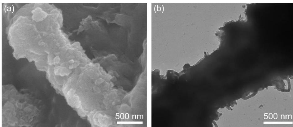
**Fig. S12** (a) SEM and (b) TEM images of the CWE FeS<sub>2</sub> after 100 cycles at 1 A g<sup>-1</sup>.
