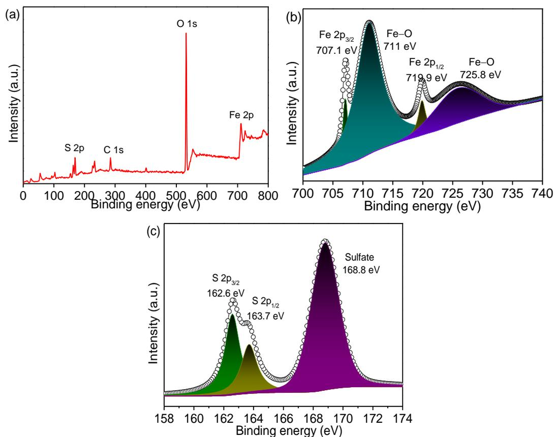
**Fig. S6** (a) XPS survey spectrum. High-resolution spectra of (b) Fe 2p and (c) S 2p of FeS<sub>2</sub>.
