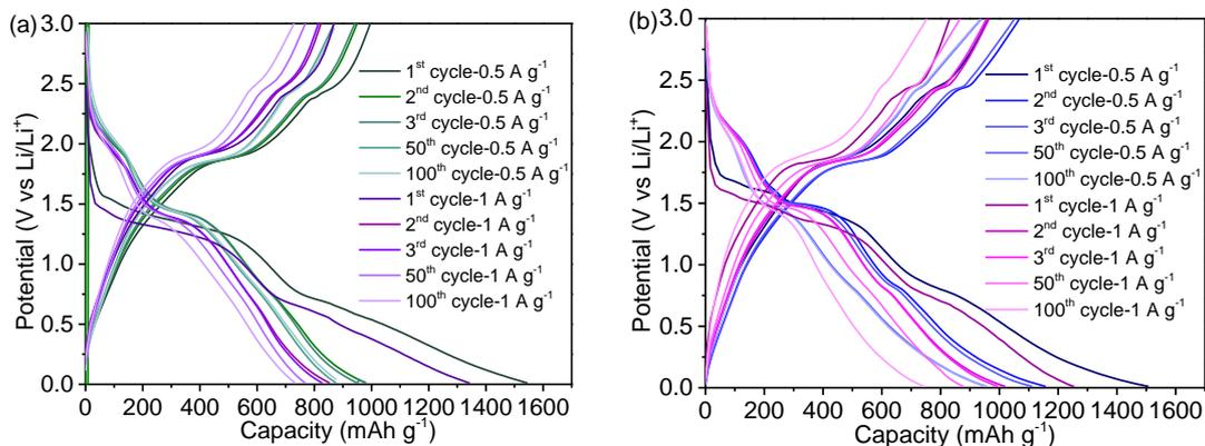
**Fig. S9** Charge-discharge curves of the CWE FeS<sub>2</sub> at rates of 0.5 and 1 A g<sup>-1</sup> under different temperatures: (a) -10 °C and (b) 45 °C.
