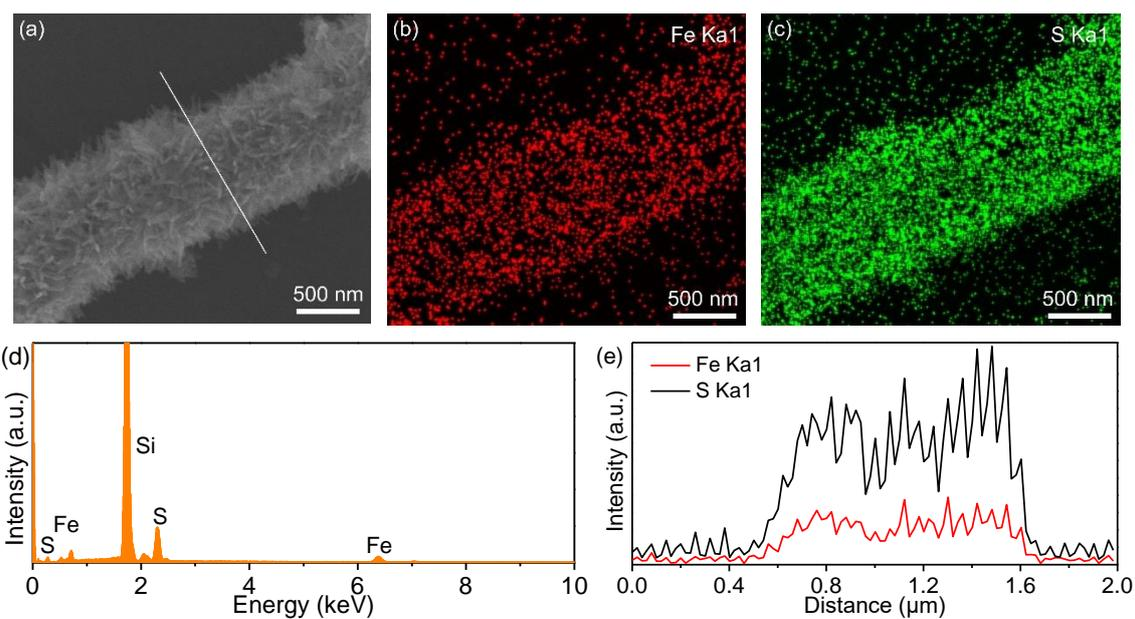
**Fig. S5** (a) SEM and (b,c) elemental mapping images of the CWE FeS<sub>2</sub>. (d) EDS spectrum. (e) The line-scanning profiles.
