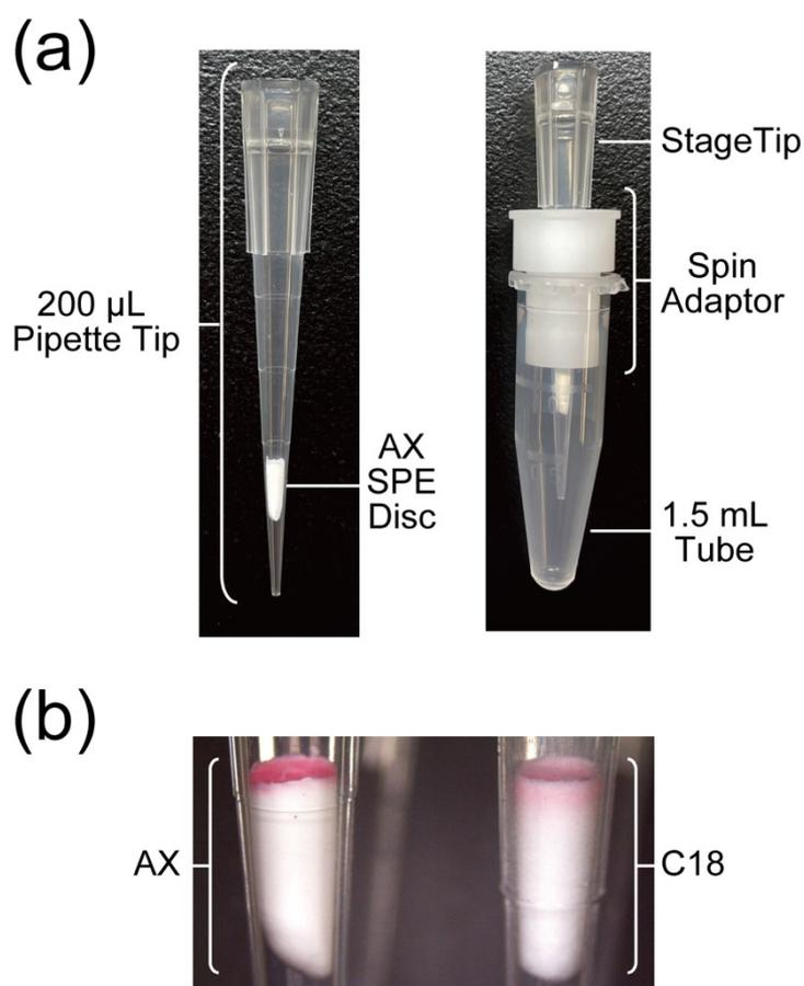
**Fig. S1** (a) Self-made AX StageTip. The StageTip used in this study was prepared by packing a single Empore anion disc (6 mm in diameter) in a 200  $\mu$ L size disposable pipette tip. Disc fitting was done manually using an Eppendorf Combitips Plus<sup>®</sup> 10 mL piston. (b) After loading 2  $\mu$ g  $\beta$ -phycoerythrin: AX SPE disc (AX) and C18 RP SPE disc (C18).
