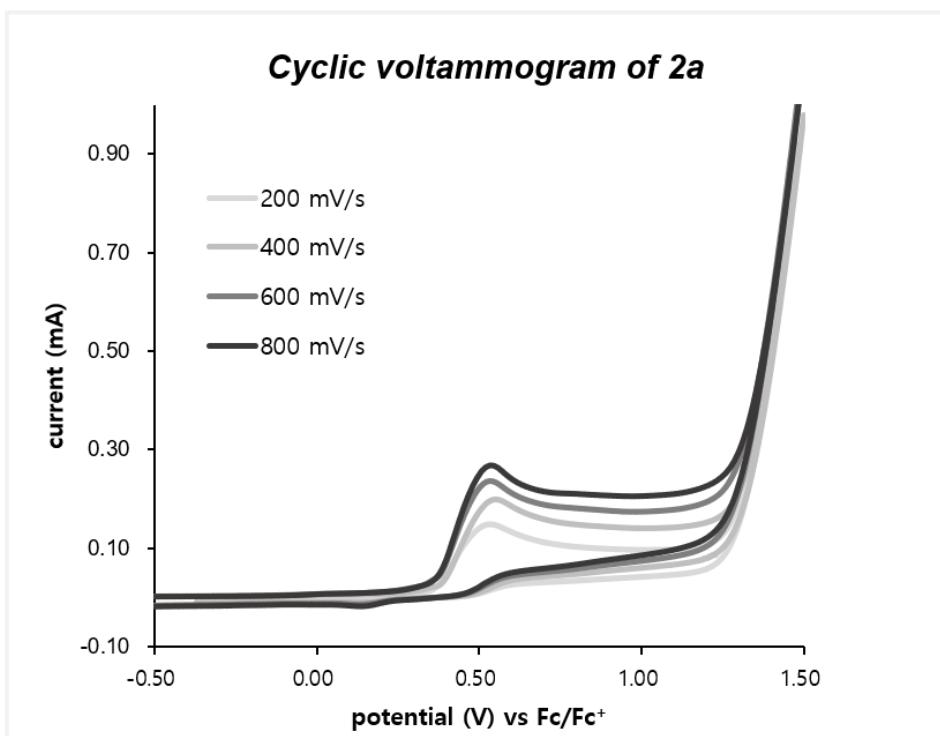
**Figure S12.** CVs of **2a** at various scan rates
