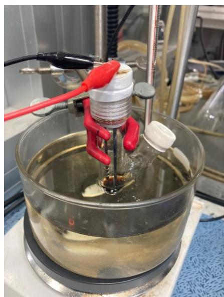
**Figure S1.** Setup for electrochemical intramolecular dehydrogenative C–H/N–H coupling
