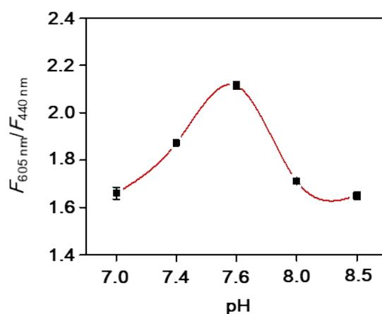
**Fig. S11.** Effect of pH on the fluorescence intensity ratio  $F_{605 \text{ nm}}/F_{440 \text{ nm}}$  of dual-recognition Van-MB-Cdots (3.0  $\mu\text{g}/\text{mL}$ , determined by Cdots) together with  $10^8$  CFU/mL of MRSA in Tris-HCl buffer (20.0 mM, 100.0 mM of  $\text{K}^+$ , 2.0  $\mu\text{M}$  of NMM). The fluorescence data were obtained with the single-excitation wavelength of 390 nm. Error bar expressed the deviation of three measurements.
