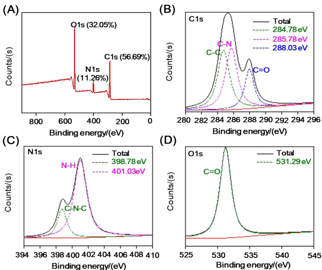
Fig. S3. XPS analysis of the as-prepared Cdots. (A) XPS, (B) C1s, (C) N1s, and (D) O1s spectra of the as-synthesized Cdots.
