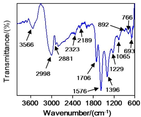
**Fig. S4.** FT-IR spectrum of the as-prepared Cdots.
