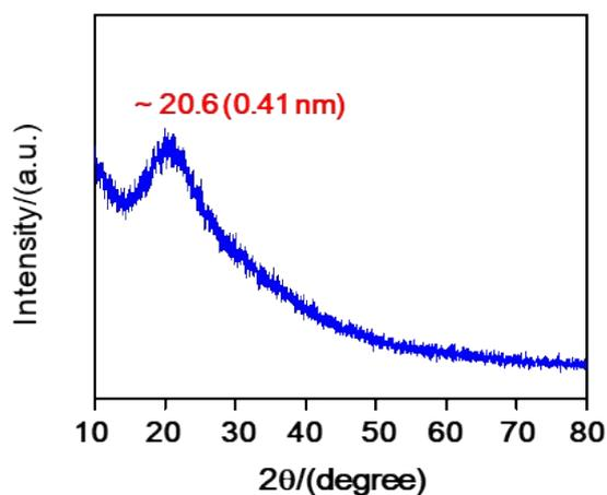
Fig. S2. XRD pattern of the as-prepared Cdots.
