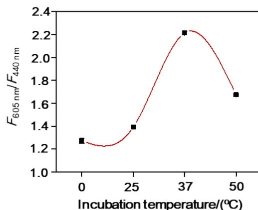
**Fig. S12.** Effect of incubation temperature on the fluorescence intensity ratio  $F_{605\text{ nm}}/F_{440\text{ nm}}$  of dual-recognition Van-MB-Cdots (3.0  $\mu\text{g/mL}$ , determined by Cdots) together with  $10^8$  CFU/mL of MRSA in Tris-HCl buffer (20.0 mM, 100.0 mM of  $\text{K}^+$ , 2.0  $\mu\text{M}$  of NMM). The fluorescence data were obtained with the single-excitation wavelength of 390 nm. Error bar expressed the deviation of three measurements.
