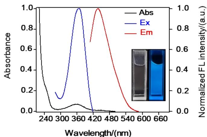
**Fig. S5.** Absorption, fluorescence emission and excitation spectra of the as-prepared Cdots in D.I. water. Inset: the photographs of the as-synthesized Cdots before (left) and after (right) excitation of a 365 nm UV lamp.
