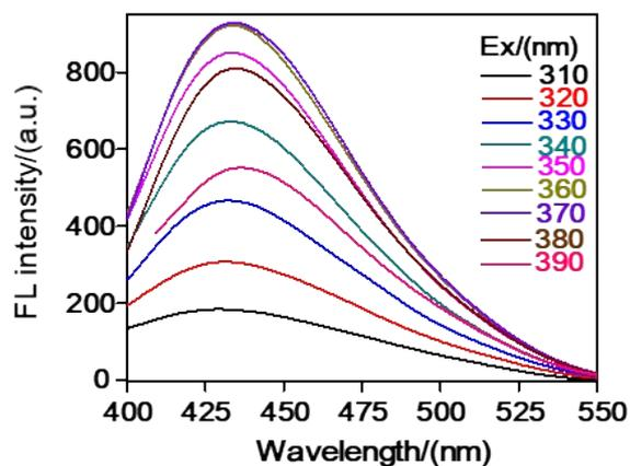
**Fig. S6.** Fluorescence emission spectra of the as-synthesized Cdots in D.I. water at different excitation wavelengths.
